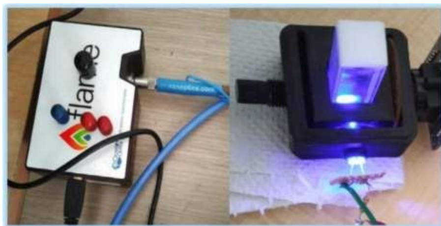
Figure 2.2 Instrumental setup of OFS
