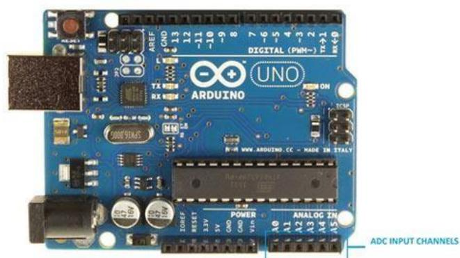
**Fig. 3.1.** Arduino Uno board.
