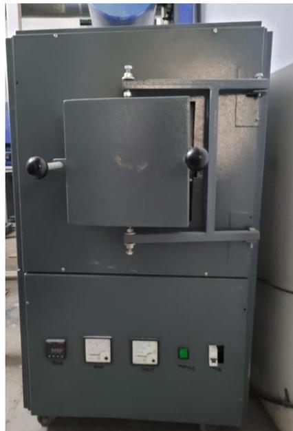
**Figure 2.4 Muffle Furnace used for annealing the prepared samples**
