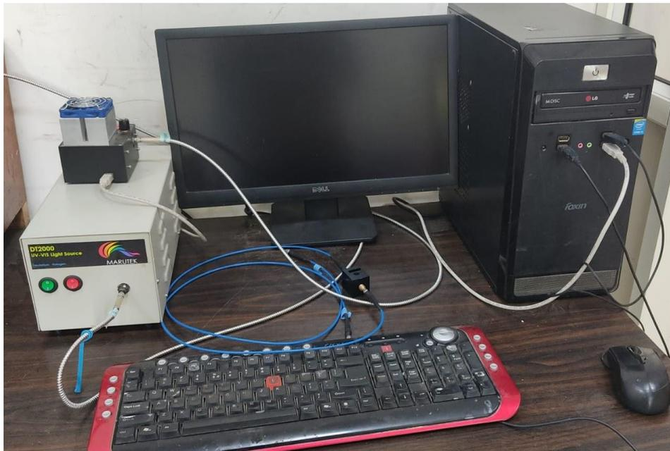
**Figure 2.11 Experimental Set-up for UV-Visible Spectrophotometer**
