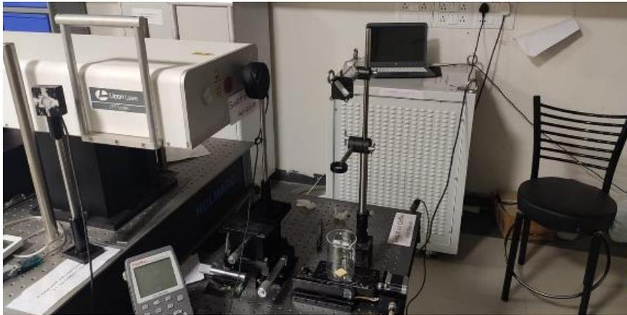
**Figure 3.3 Laser Shock Peening Setup**
