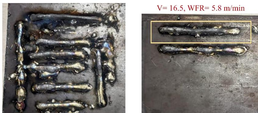
**Figure 4.1 Track deposition for parameter optimization**
