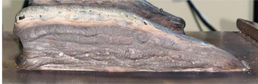
Figure 4.6 Incremental Gradient Structure wfs 3.0 m/min FGM of SS316L and IN625
