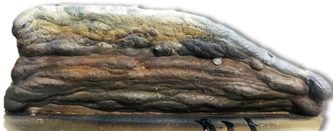
Figure 4.5 Incremental Gradient Structure wfs 4.0 m/min FGM of SS316L and IN625
