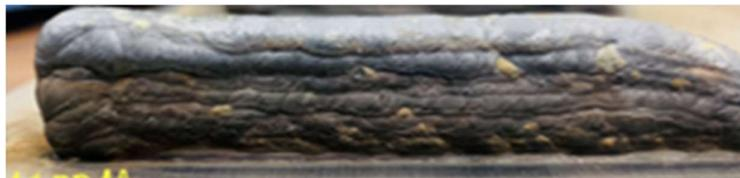
Figure 4.10 Sandwich AABB gradient structure of FGM
