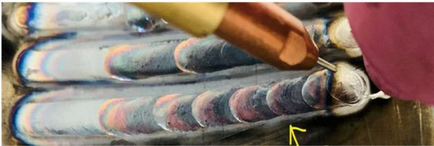
(c)  $I=170A$ ,  $V=200\text{mm}\backslash\text{min}$ ,  $wfs=0.4\text{m}/\text{min}$
