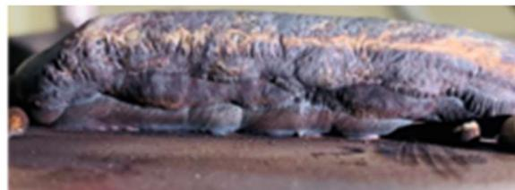
Figure 4.11 Sandwich ABAB gradient structure of FGM
