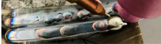
(a)  $I=170A$ ,  $V=200\text{mm}\backslash\text{min}$ ,  $wfs=0.2\text{m}/\text{min}$
