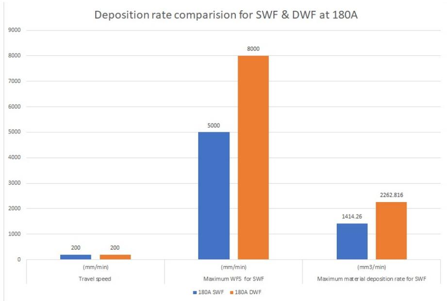
Fig. 4.29 Deposition rate comparison for SWF & DWF at 180A current
