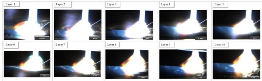
*Fig. 4.4 Melt pool diagram at 180 A current at 5 m/min WFS*
