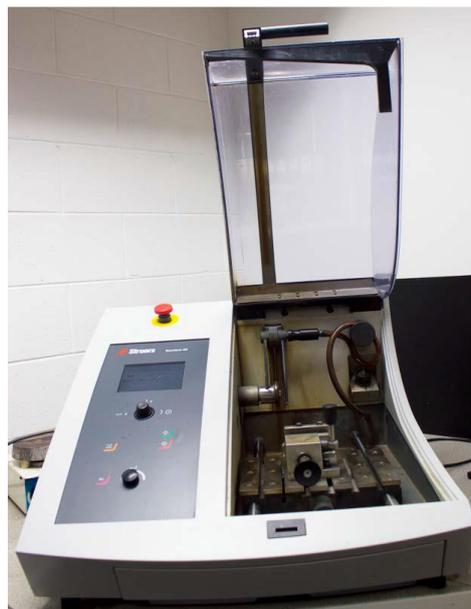
**Fig. 3.3.** Setup of high-speed cutter
