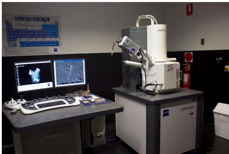
**Fig. 3.4.** Setup of Scanning Electron Microscope [25]
