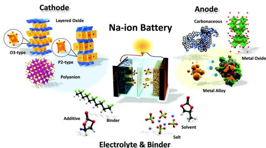
**Figure 1.6** Schematic showing sodium ion battery cathode, anode, and electrolyte[27].
