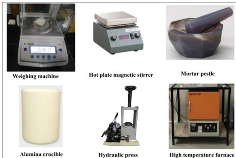
Figure 2.2. The apparatus used in ceramic fabrication.
