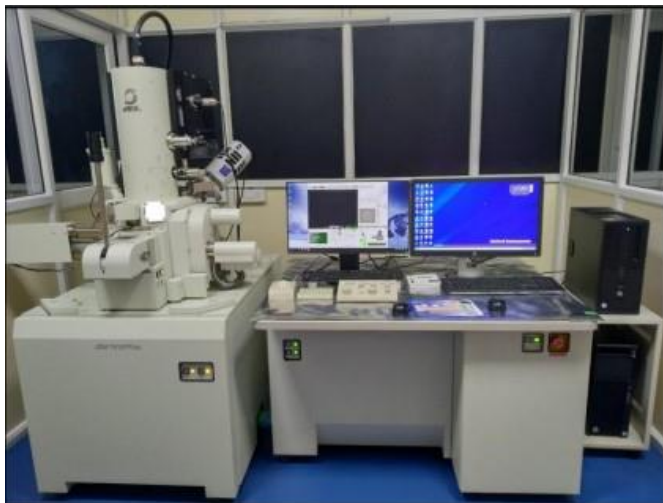
Figure 2.6. The JEOL-7610 Field Emission Scanning Electron Microscope.
