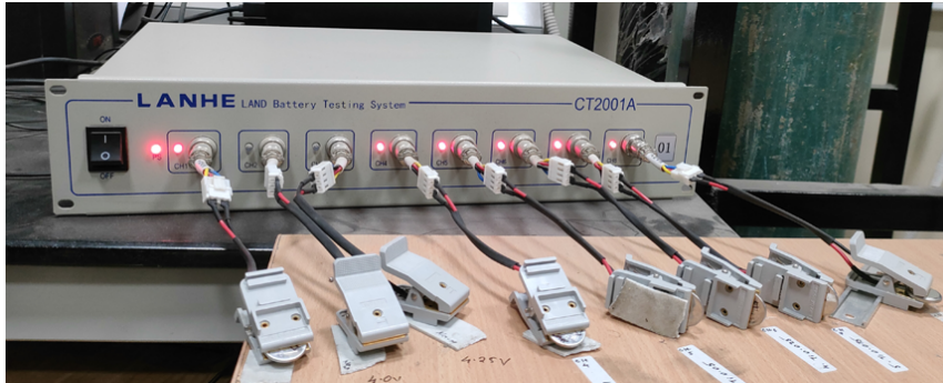
Figure 2.8 The LANHE battery tester.
