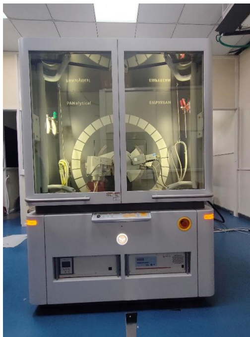
Figure 2.5. The Malvern Pananalytical diffractometer.
