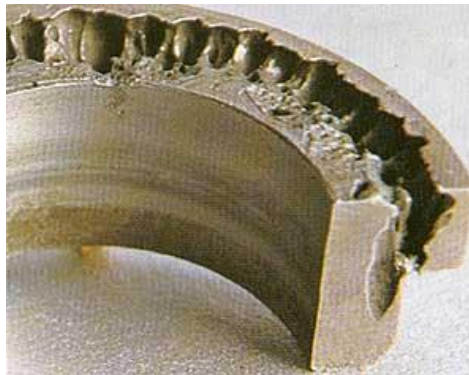
Fig 5 - Failure due to Intergranular corrosion
