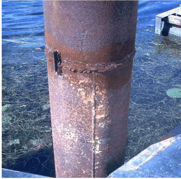
Fig 1 - Uniform corrosion of pipe in seawater[47]
