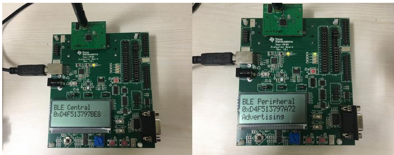
Figure 3.3 Smart RF Boards-BLE peripheral and BLE central
