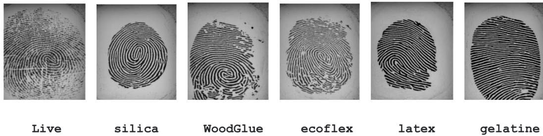
FIGURE 1.2: Live and fake fingerprint images created with different spoof materials.
