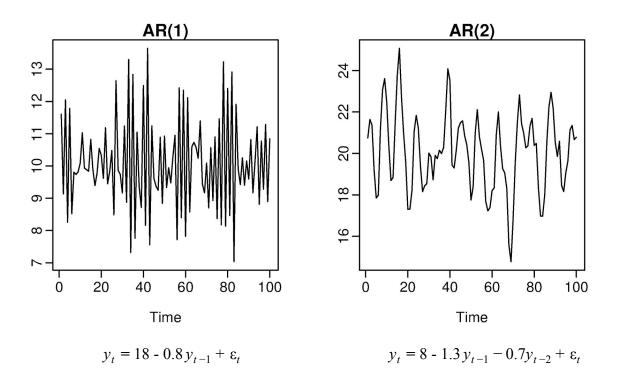
Fig: Two examples of data from autoregressive models with different parameters. Left: AR(1). *Right:* AR(2) with In both cases,  $\boldsymbol{\varepsilon}_t$  is normally distributed white noise with mean zero and variance on
