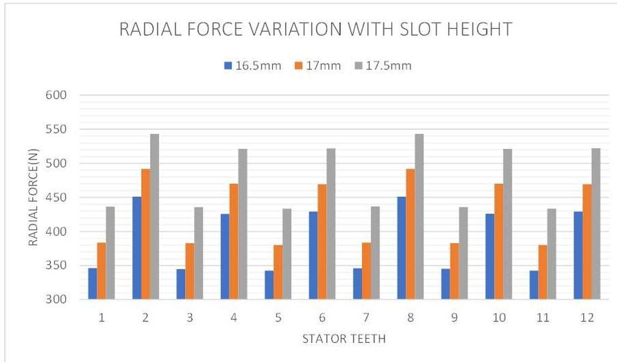
Fig 10: radial force variation with slot height.
