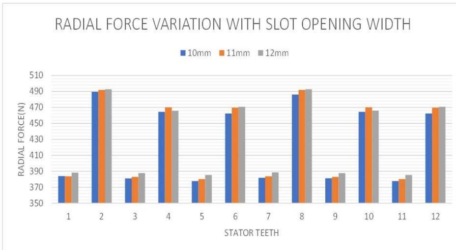
Fig 11: radial force variation with slot opening width.
