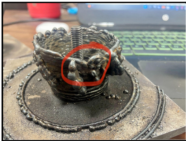
Figure 20: Gaps between the deposited layer
