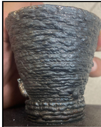
Figure 25: No material getting deposited on outer surface
