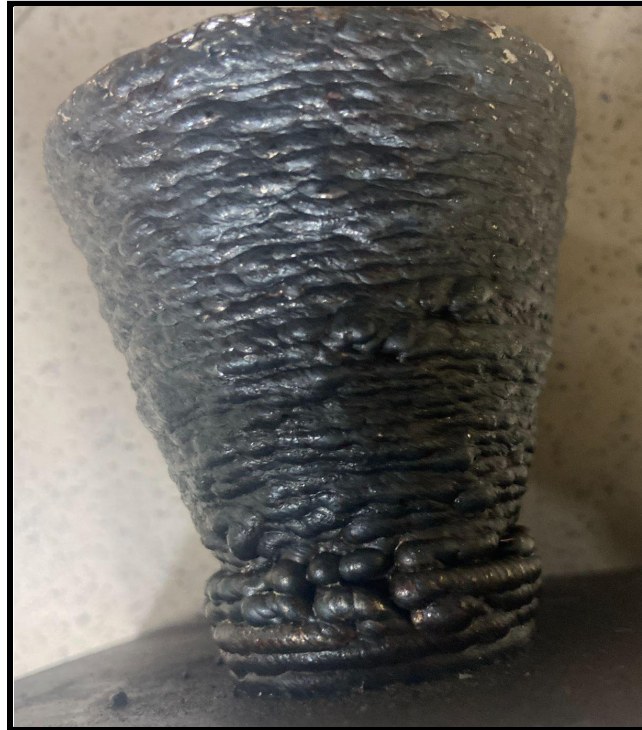
Figure 27: 4- Double layers deposited to give offset
