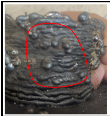
Figure 24: Material Getting deposited on the outer surface of cone
