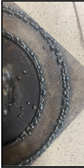
Figure 28: Uneven bead formation for circles with larger diameter
