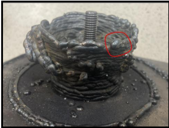
Figure 22: Bumps at the top surface
