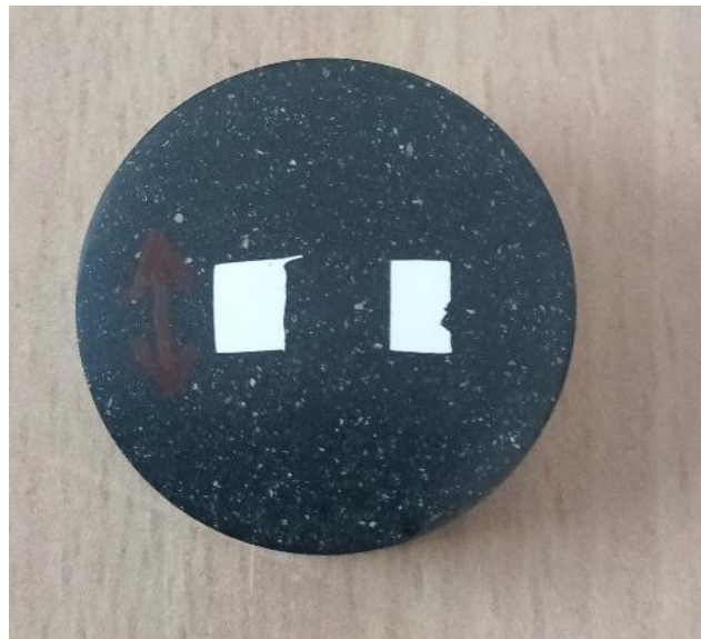
Figure 6.3: Hydrogen charged specimens for Microstructure, Hardness and XRD analysis
