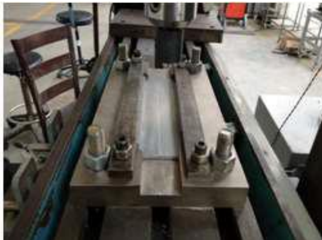
Figure 6.5: Setup showing plates about to be welded
