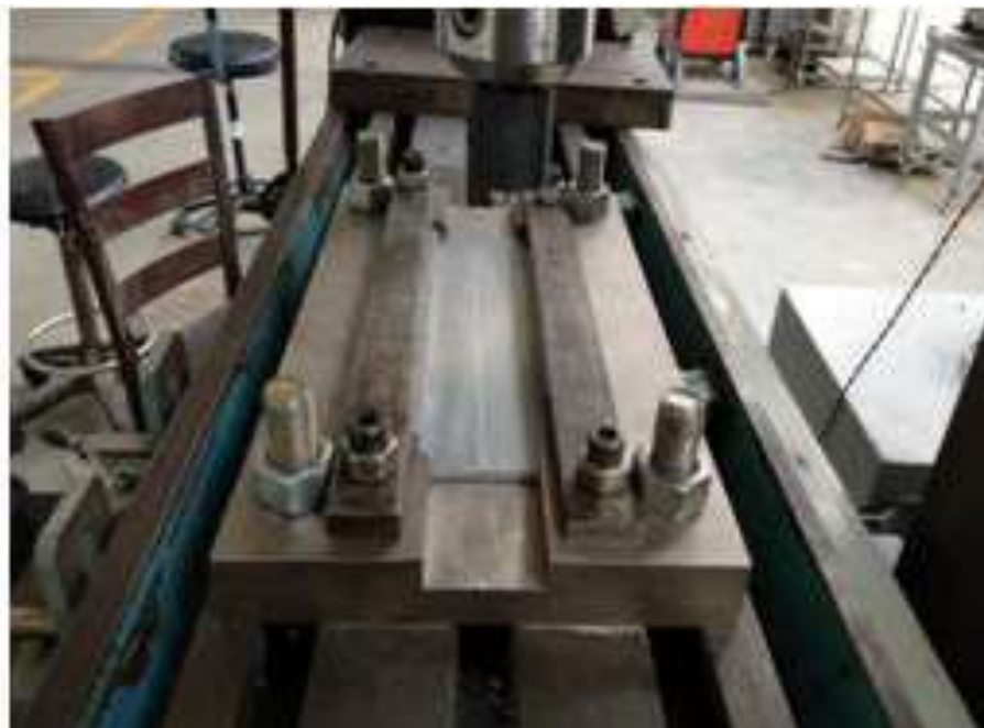
Figure 1.1: Friction stir welding fixture at IITI central workshop
