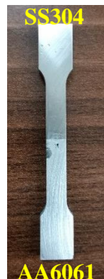
Figure 6.7: Tensile test specimen of AA6061-SS304 weld joint
