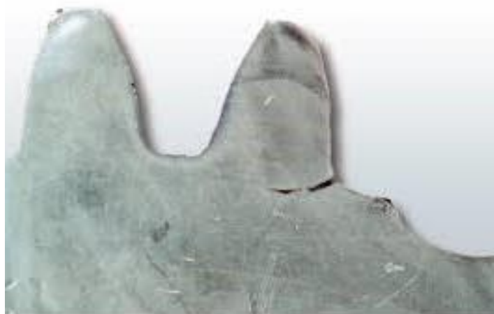
Figure 2.4: Fatigue crack in gear tooth root fillet
