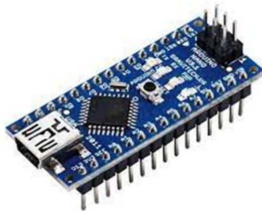
Figure 6.4: Arduino nano V3.0
