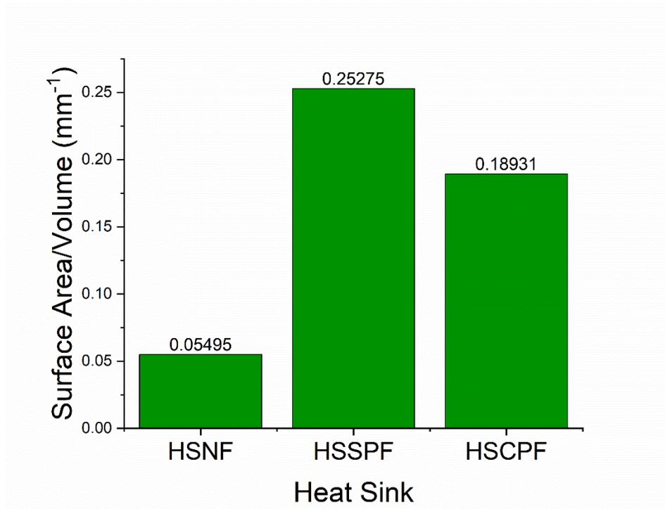
**Fig. 17 Surface area per unit volume comparison of HSNF, HSSPF, and HSCPF**
