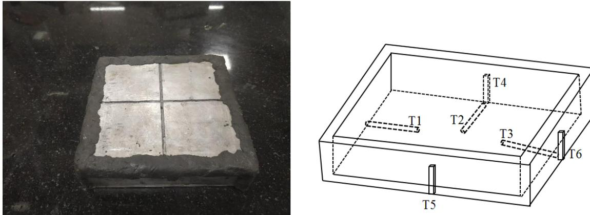
**Fig. 6 Grooves in Heat Sinks for placing thermocouples**
