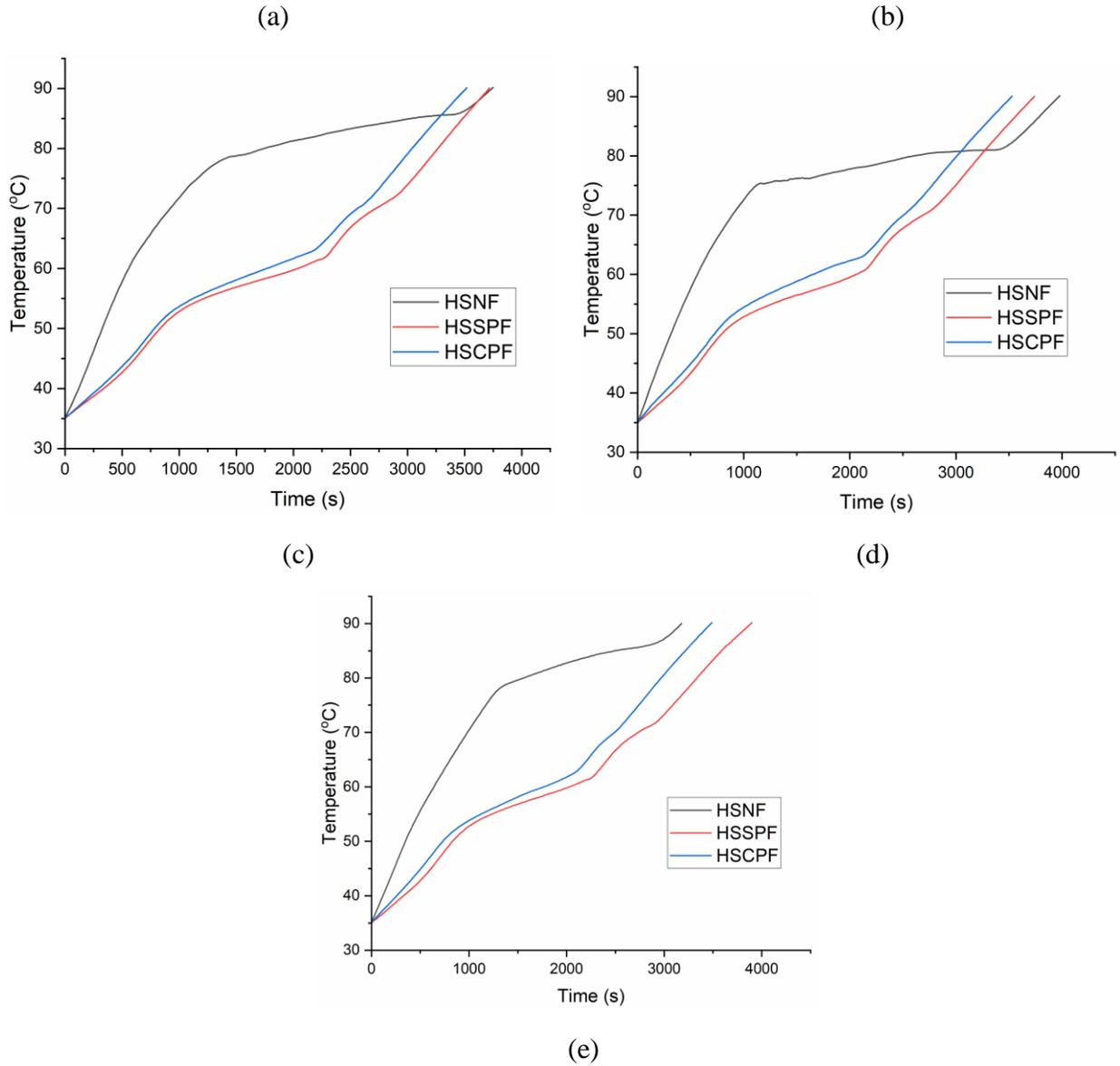
**Fig. 14 Variation of base temperature with each concentration of nanoparticles in different HS (a) Pure PCM (b) 0.5% Al<sub>2</sub>O<sub>3</sub> (c) 1% Al<sub>2</sub>O<sub>3</sub> (d) 0.5% CuO (e) 1% CuO**
