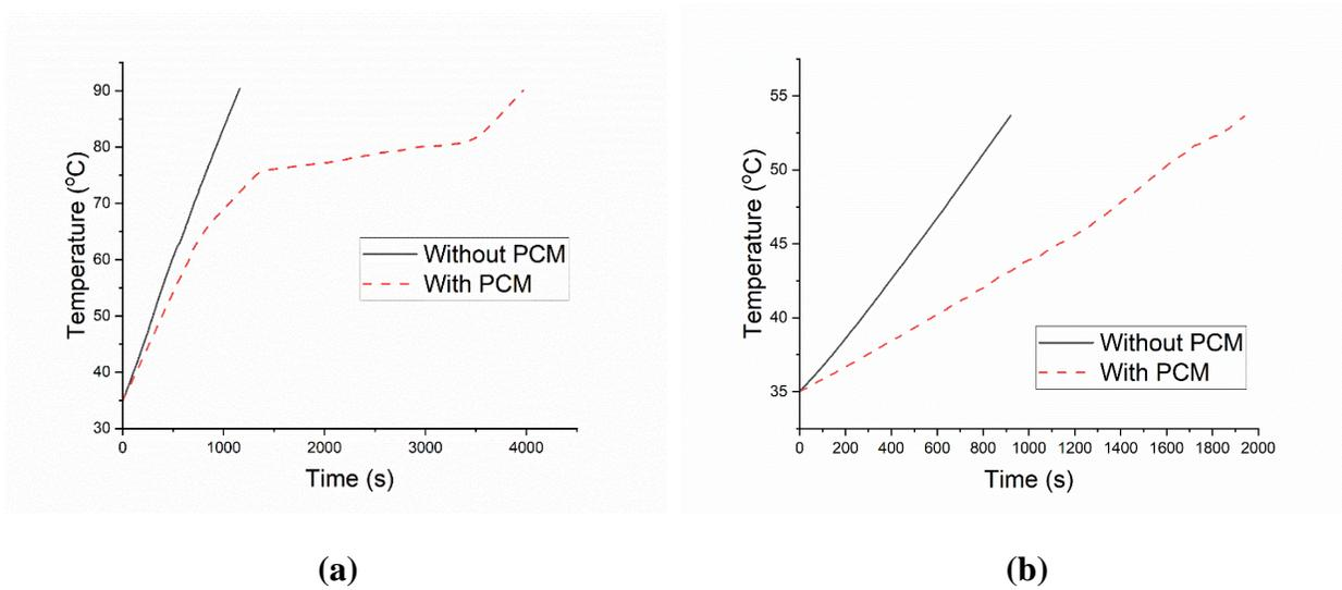
**Fig. 10 Comparison of variation of (a) base temperature and (b) Side wall temperature of HS with PCM and Without PCM**
