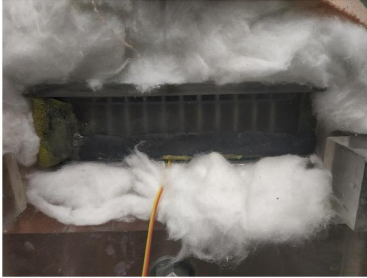
**Fig. 13 HS filled with liquid PCM**
