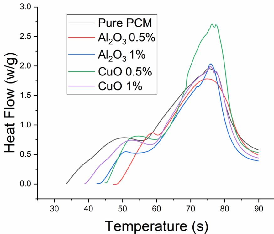
Fig. 8 Heating curve for NePCM
