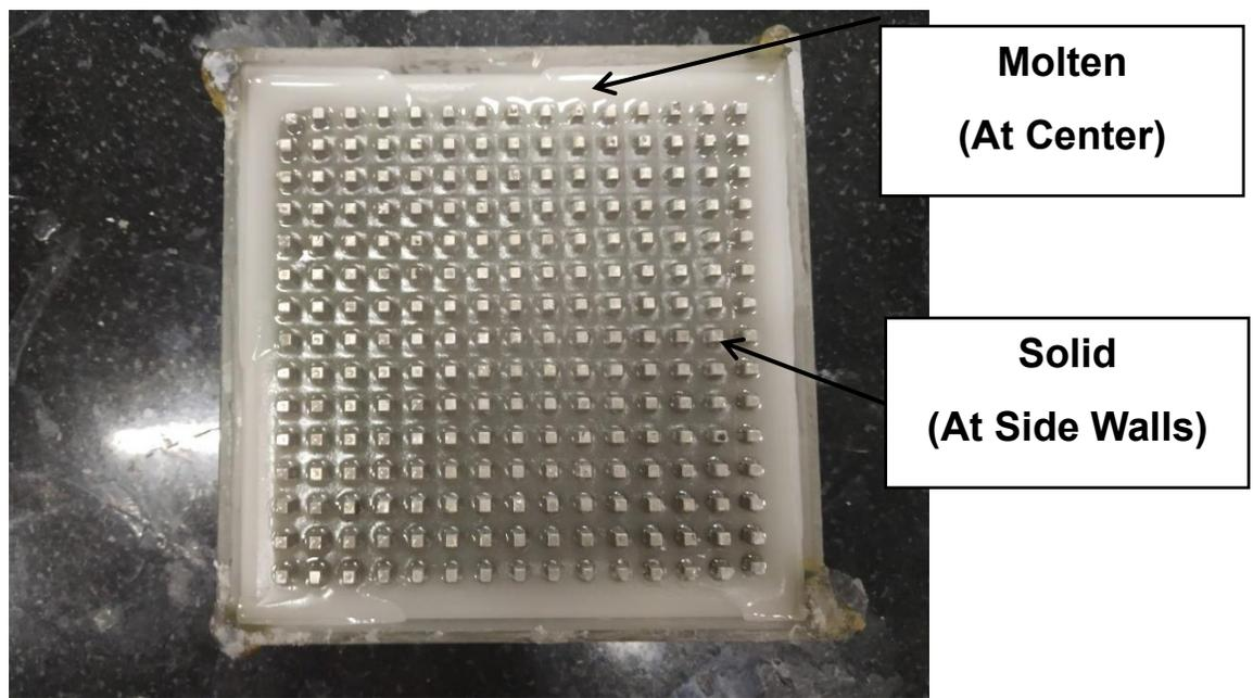
**Fig. 12 PCM in latent melting phase**
