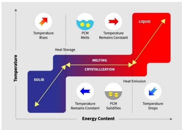
**Fig. 1** Ideal heating and cooling curve of PCM for thermal management system
