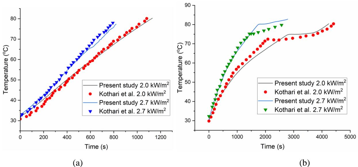
**Fig.9 Validation of Experimental setup with (a) HS without PCM (b) HS with PCM**
