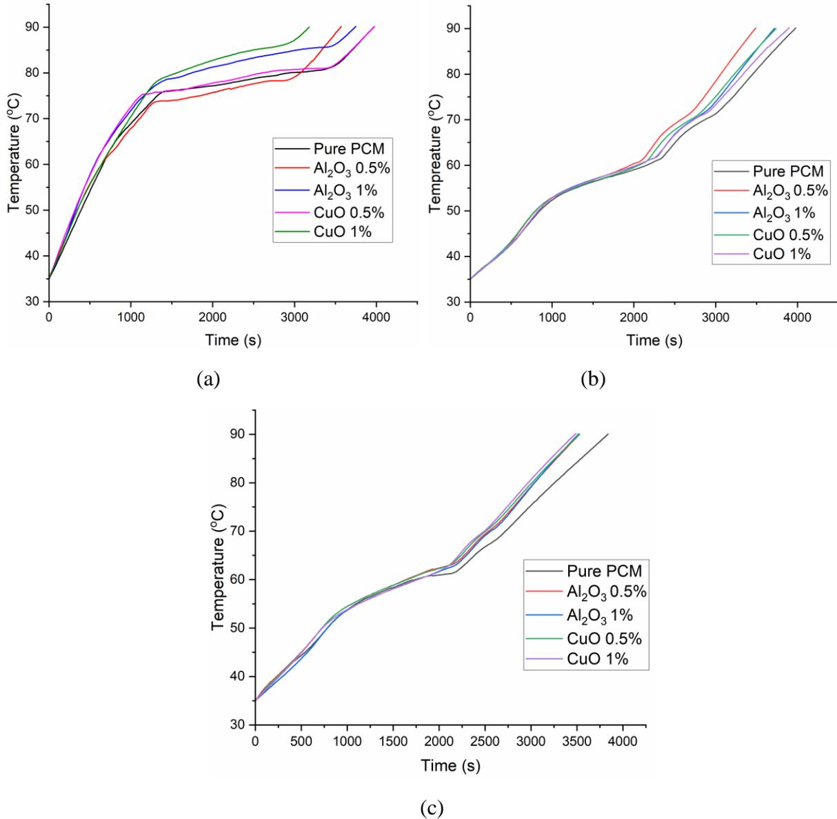
**Fig.15 Variation of base temp. for each HS with (a) HSNF (b) HSSPF (c) HSCPF**
