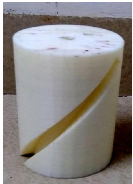
Figure 12: 3-D printed model of inner cylinder
