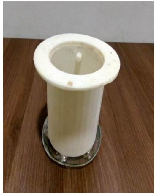
Figure 14: 3-D printed model of outer cylinder
