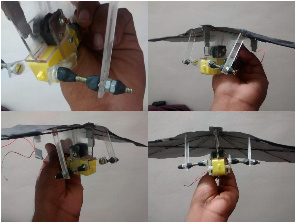
Fig. 12 - Dual-shaft motor based flapping mechanism
