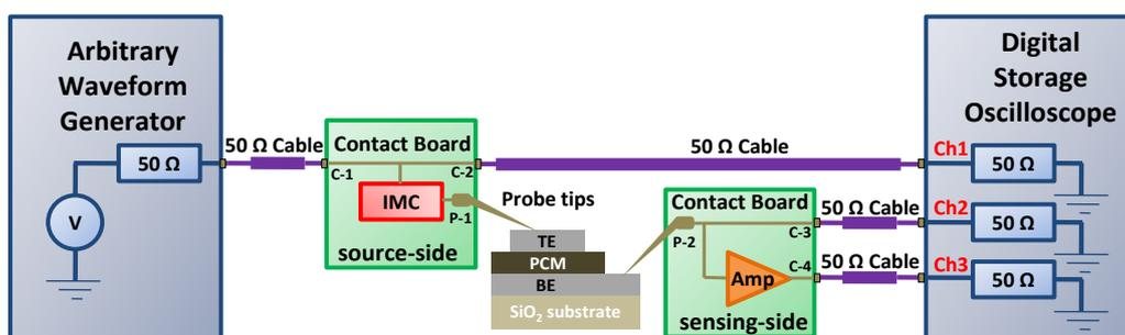
**Figure 3.** Schematic of the custom-designed PET setup.
