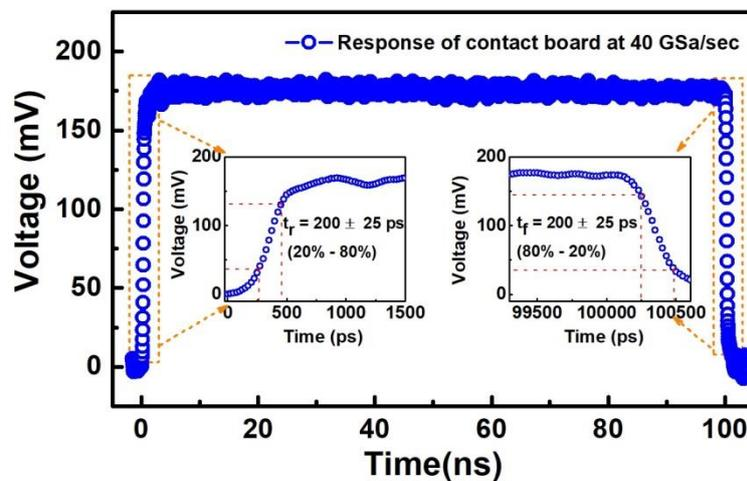
**Figure 4.** The output response of the high-frequency contact boards for the standard test pulse (STP).
