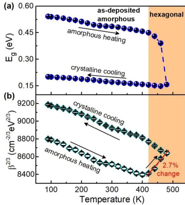
**Figure 6.** Temperature-dependence of (a) band gap  $E_g$  and (b) short-range disorder measured by the Tauc parameter  $\beta^{2/3}$ .
