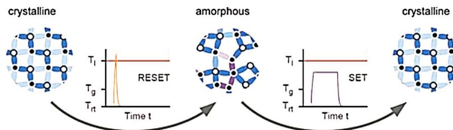
**Figure 1.** Principle of operation of Phase change memory technology [5].
