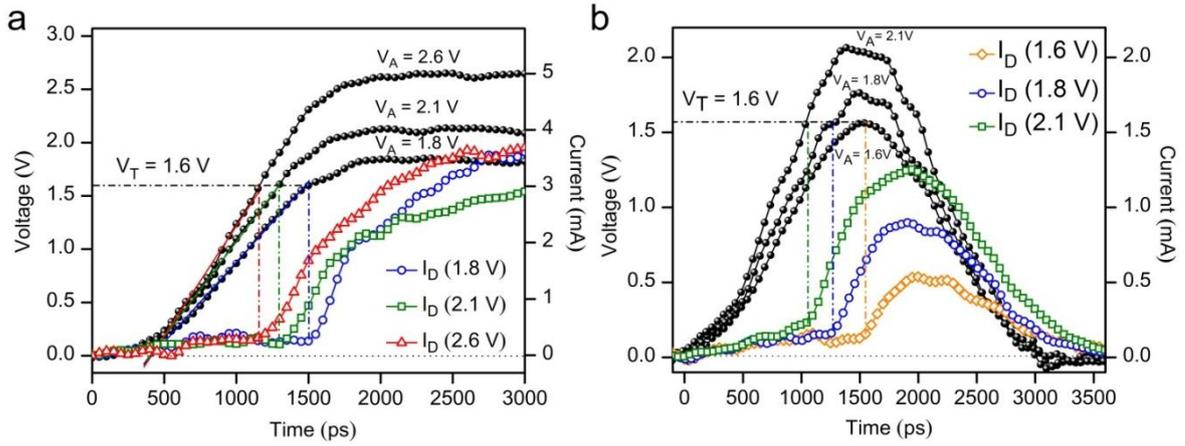
**Figure 5.** Transient responses for different  $V_A$  of 1.8 V, 2.1V and 2.6V (a) for pulse having the rise time of 1 ns, fall time of 100 ns and pulse width of 100 ns. (b) for a pulse having the rise and fall time of 1 ns with the pulse width of 1.5 ns (FWHM).
