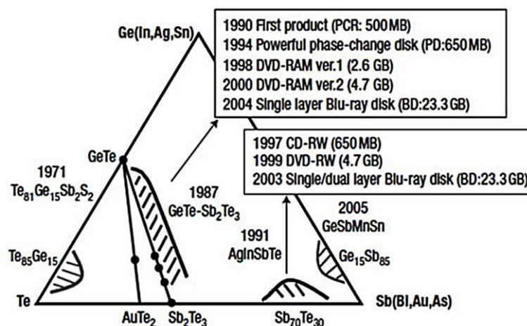
**Figure 2.** Ternary phase diagram of the phase change memory material families [2].
