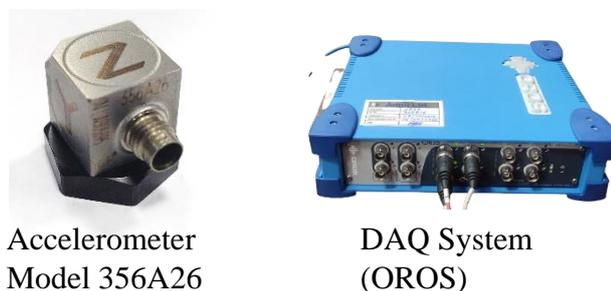
*Figure 4.5 Major components and accessories of the accelerometer*
