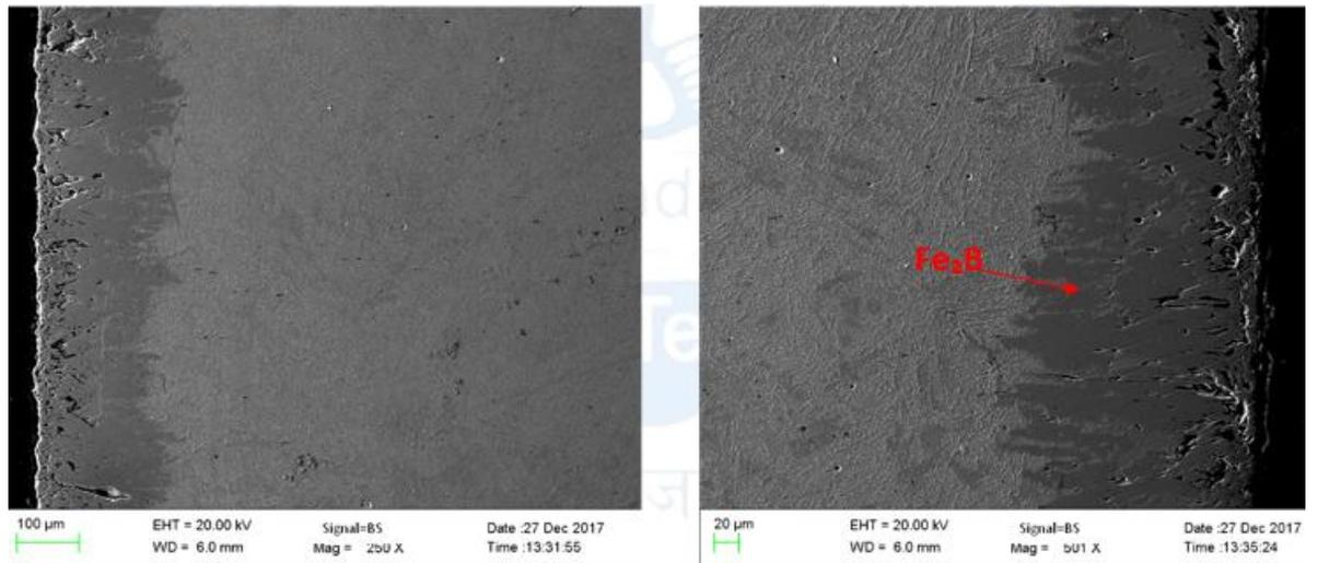
**Figure 5.17: SEM image showing the Morphology of boride layer in EN24 boronized at 1050°C for 4h.**
