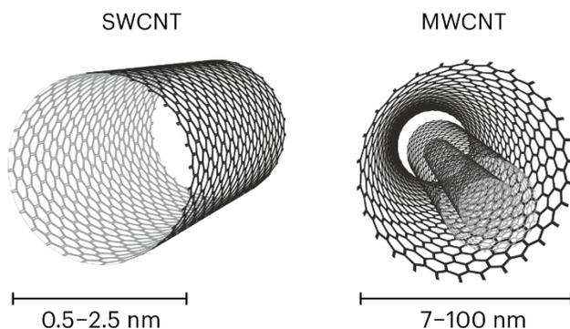
**Figure 1. Single-walled Carbon Nanotube (SWCNT) and Multi-walled Carbon Nanotube (MWCNT) [8]**
