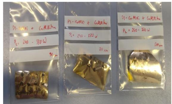
**Figure 8.1: Samples developed with selective laser melting on Kapton polyimide sheets.**
