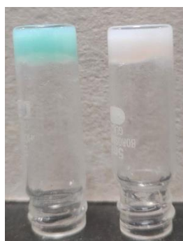
Figure 4.3: Inversion test of Cu metallo gel and organogel of A2
