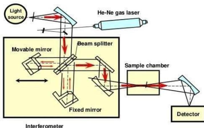
**Fig. 2.4:** Schematic of FTIR Instrument [16]
