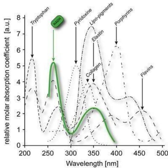
**Fig. 2.6:** Absorption Spectra of NADH [19]
