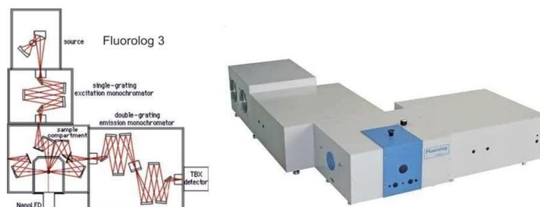
**Fig. 2.7:** Schematic of Fluorolog 3
