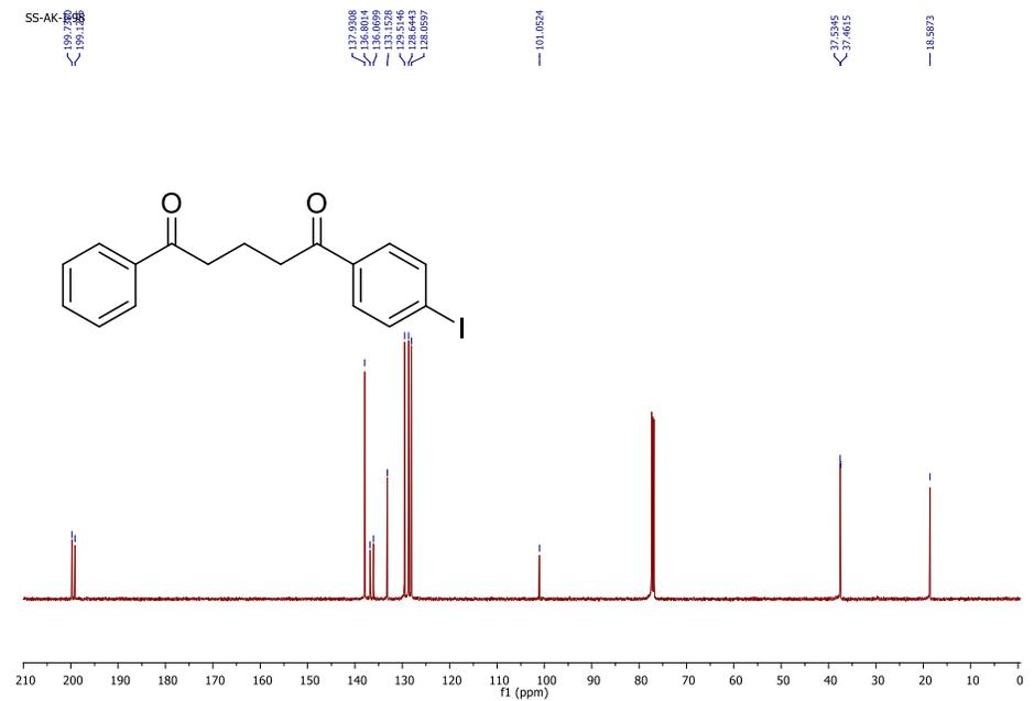
Figure 56: <sup>13</sup>C NMR spectrum (125MHz) of 3af in CDCl<sub>3</sub>
