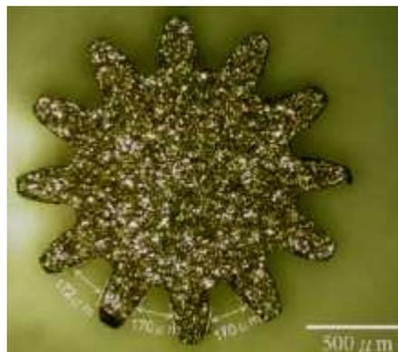
**Fig. 2.10:** SEM images of SKD11 tool steel micro-spur gear manufactured by Yan and Chiang (2009) using  $\mu$ -WSEM and 70  $\mu\text{m}$  diameter copper wire.
