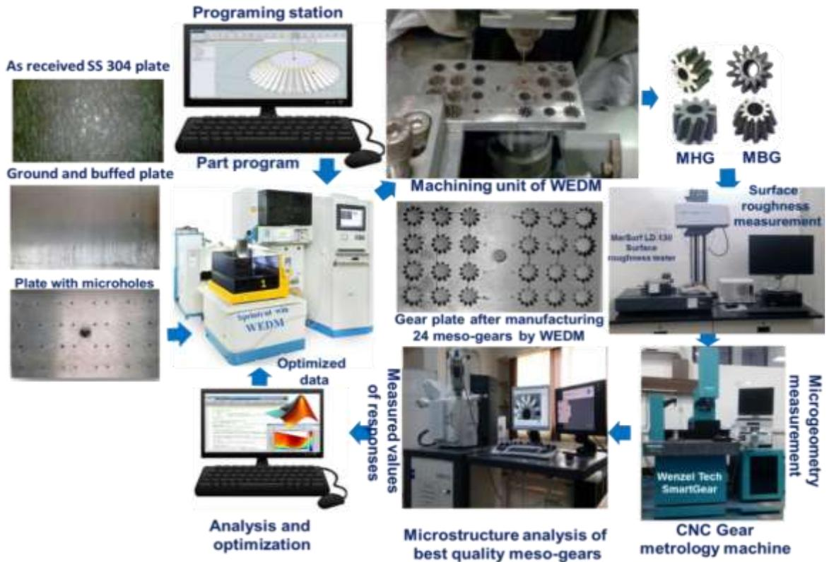
**Fig. 3:** Sequences of different activities used in manufacturing of MBG and MHG and measurements of their responses.
