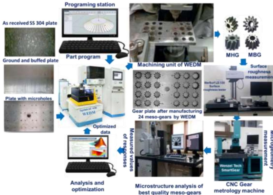
**Fig. 3.4:** Different activities and their sequence used in the experimental investigations of the present work.
