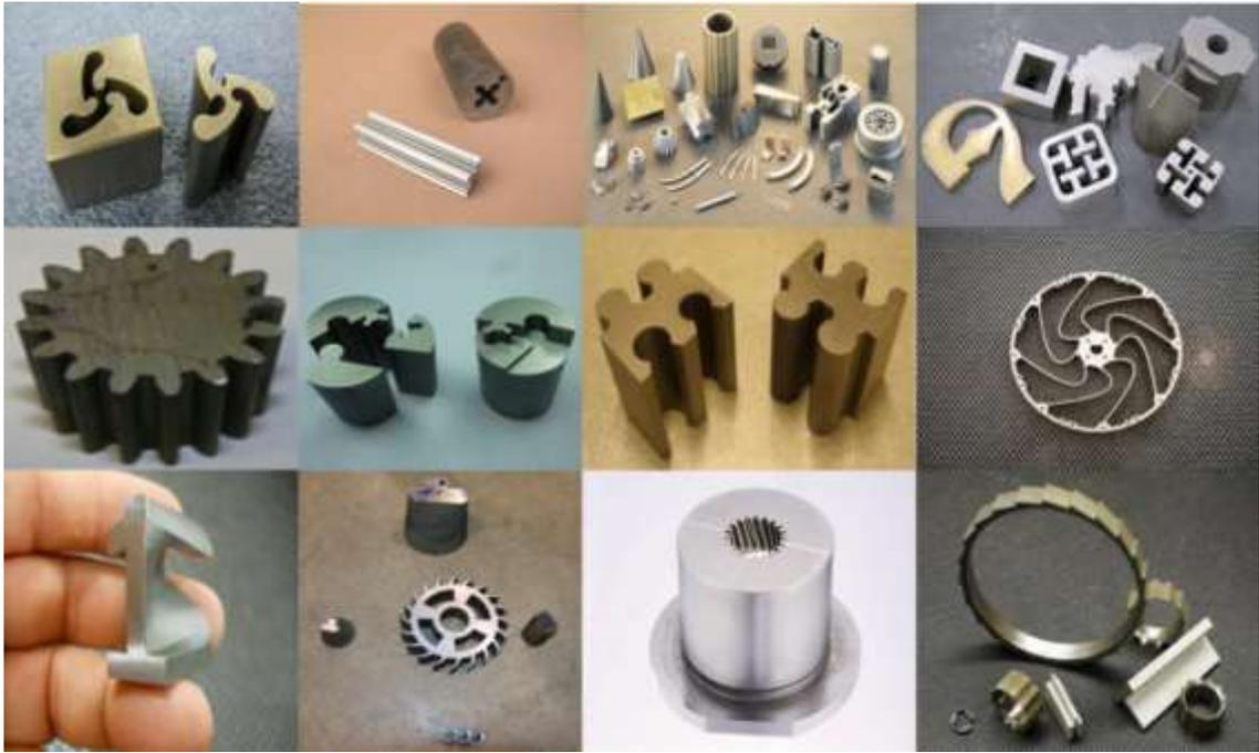
**Fig. 1.11:** Some typical complicated parts manufactured by WSEM processes.
