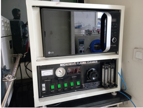
Figure 5.2: photograph showing Microwave Plasma Cleaner used for substrate cleaning
