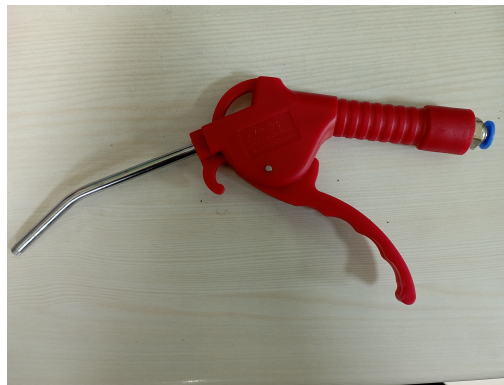
Figure 5.1: Photograph showing nitrogen gun typically used for substrate cleaning
