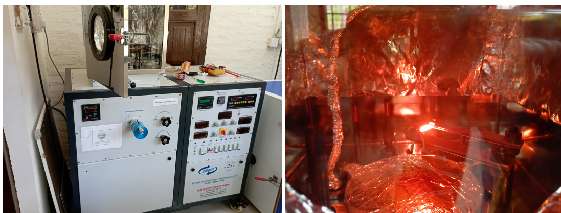
Figure 5.7: (A) Thermal Evaporation Unit. (B) Evaporating Gold on device
