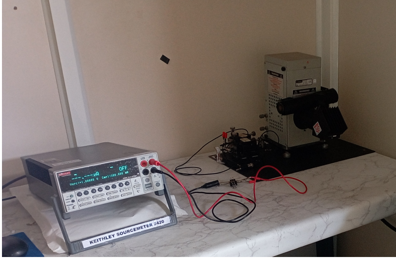
Figure 6.24: Solar Simulator setup
