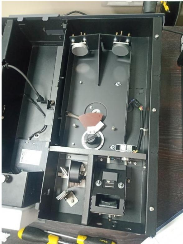
**Figure 2.5:** Experimental set up utilized for diffuse reflectance measurement, (a) Carry 60 UV-Visible Spectrometer, (b) Internal set up of UV-Visible spectrometer.<sup>60</sup>
