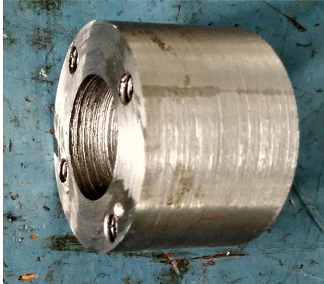
**Fig. 3.6** Image of the flange after fabrication
