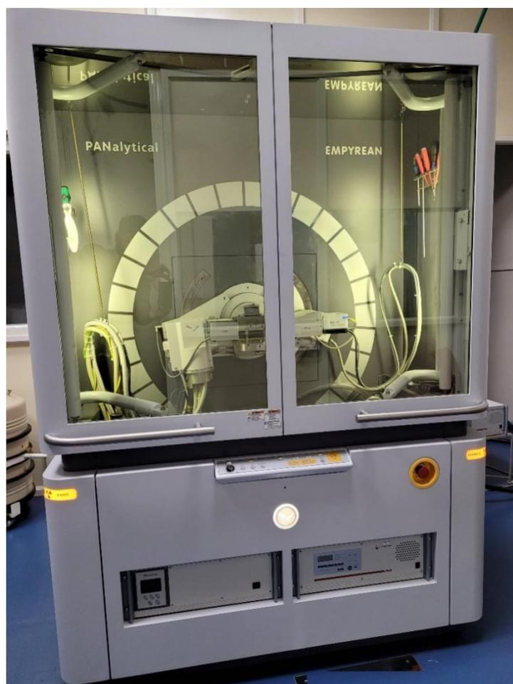
**Fig. 2.3.** Image of X-ray diffraction (XRD) instrument used in the present study.
