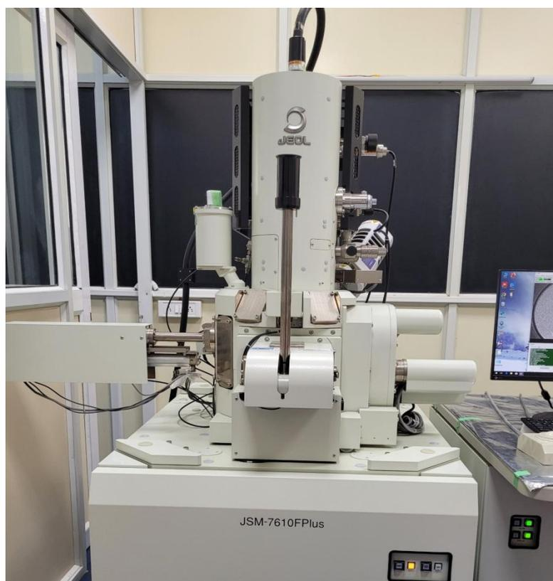
**Fig. 2.4.** Image of the FESEM instrument used in the present study.
