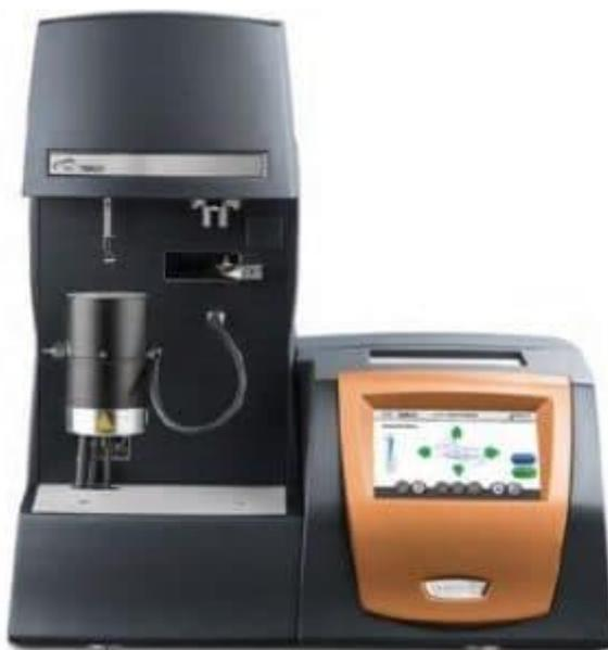
**Fig. 2.7.** Image of the equipment used for Thermogravimetric Analysis [32]
