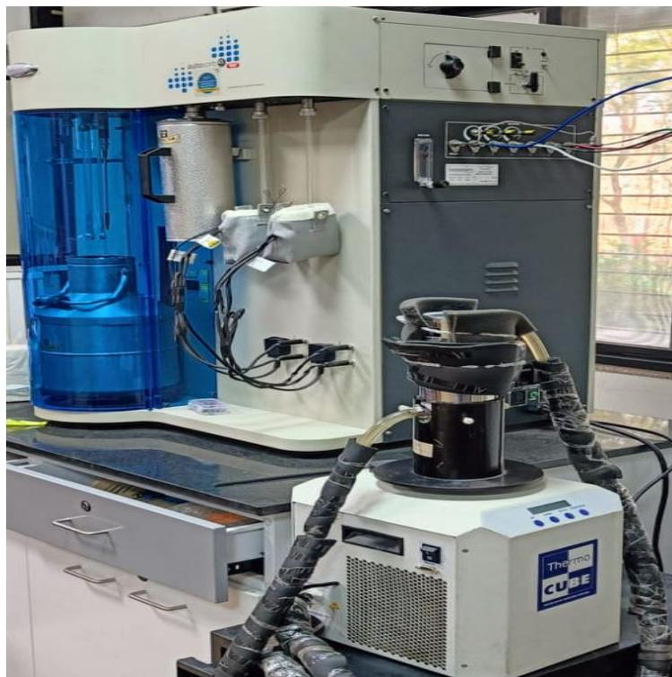
**Fig. 2.5.** Image of the BET instrument used in the present study.
