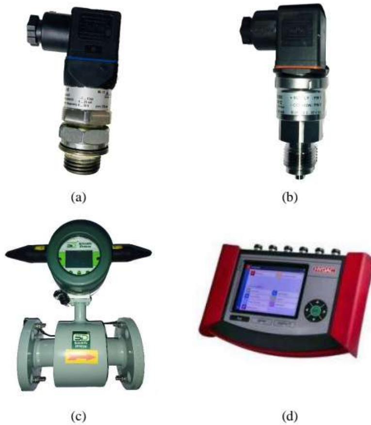
Figure 3. 4 Images of the measuring equipment used (a) Suction pressure sensor (b) Discharge pressure sensor (c) Flowmeter (d) HYDAC System
