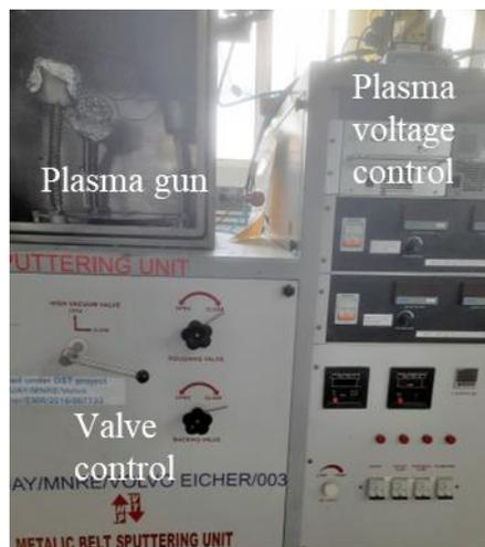
**Figure 3.5 Sputtering Deposition unit**
