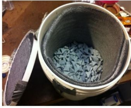
Fig. 1.8: Image showing centrifugal tumble finishing.
