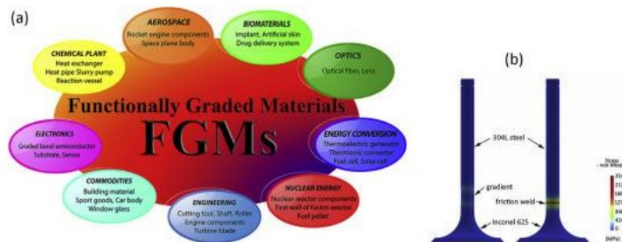
Fig. 1.1 a) The application fields of FGMs. b) Finite element analysis of a gradient transition from 304L stainless steel to Inconel 625 (left) compared to a friction-welded joint of the same materials (right) for an automobile valve stem at operating temperature 1000 K [6].
