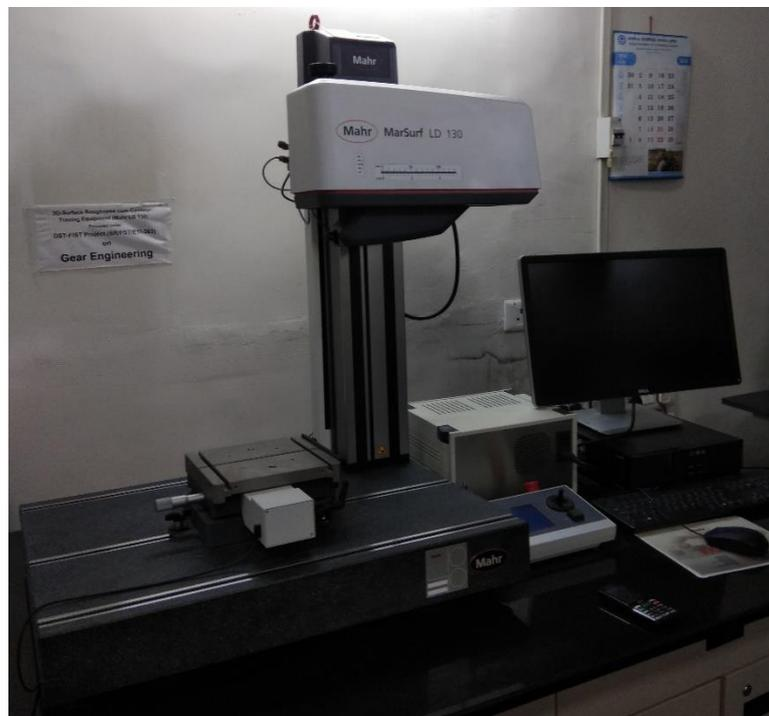
**Figure 3.8: Roughness Test Instrument**
