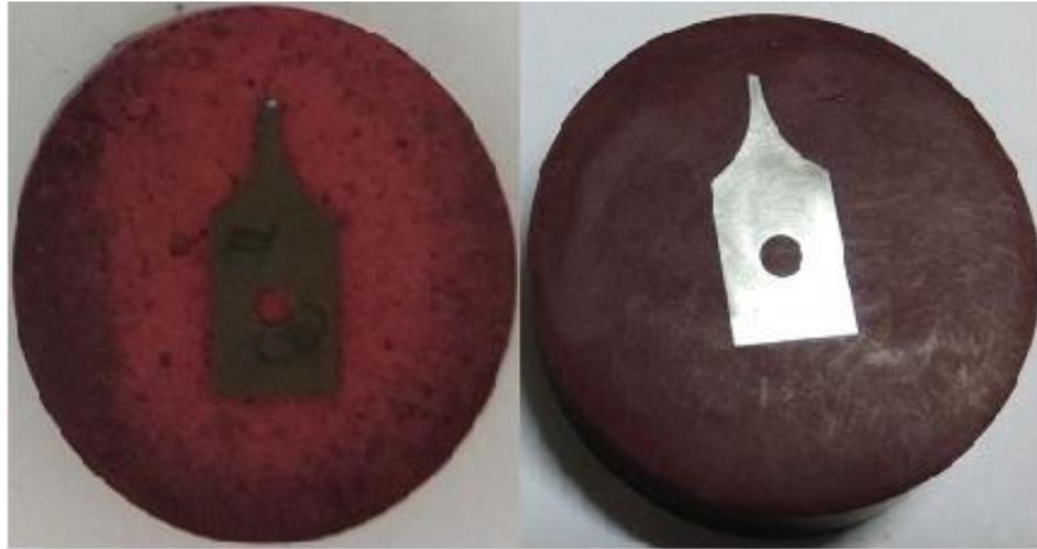
**Figure 3.3 : Mounted samples for microstructure analysis: (a) before polishing (b) after polishing**
