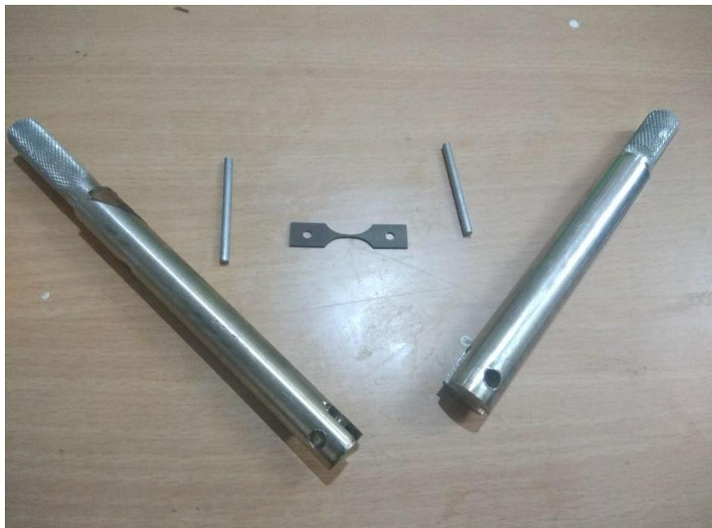
**Figure 3.5: Jigs for tensile testing**
