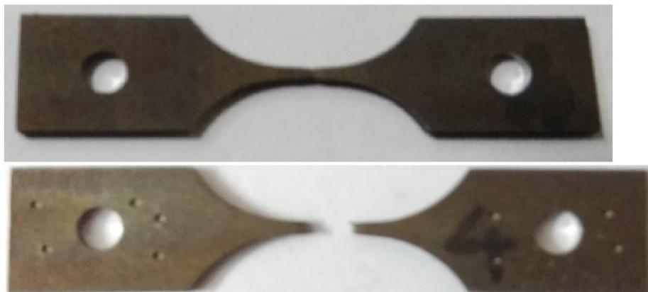
**Figure 4.2: Tensile test specimen**
