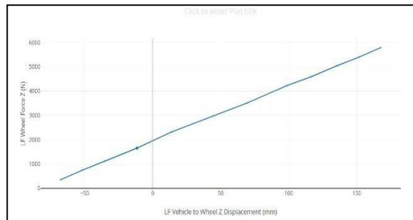
Fig 9 Wheel rate test data for front half car model
