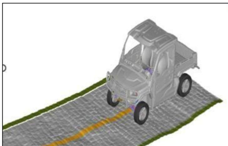
Fig 26. Virtual simulation vehicle moving on road
