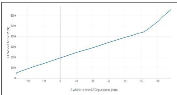
Fig 8 Wheel rate simulation Correlation for front half car model
