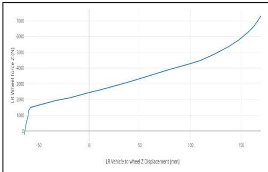
Fig 10. Wheel rate simulation
