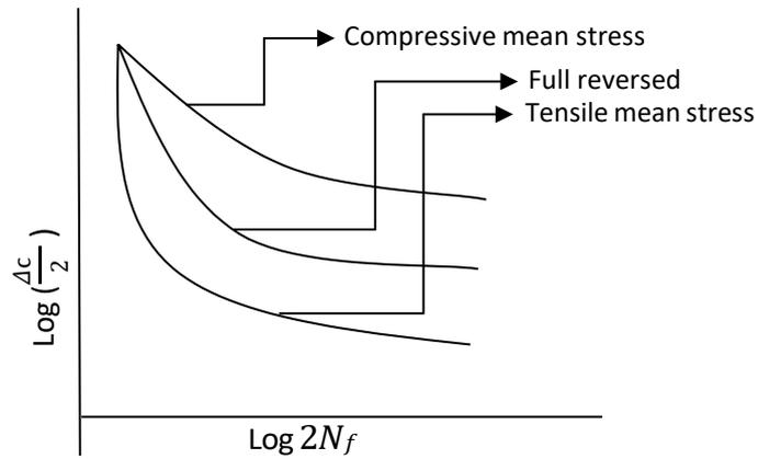
Fig.7 Effect of mean stress on strain life curve
