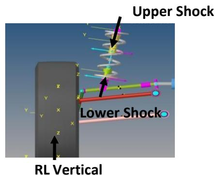
Fig 2. Suspension Geometry
