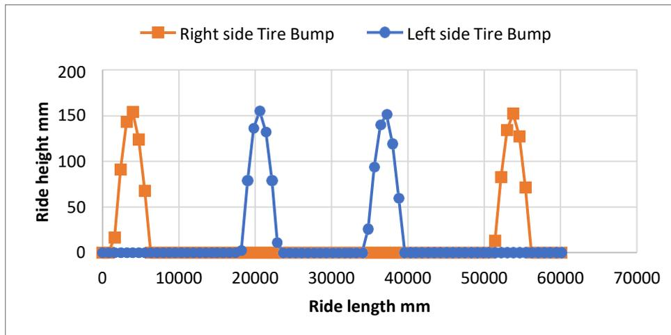
Fig13. Input Signal to Post
