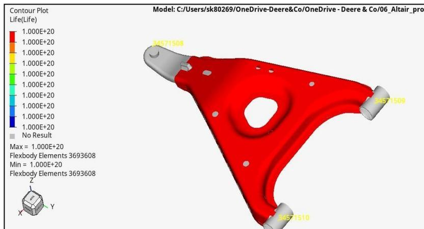
Fig 21. Npost fatigue analysis results for wheel displacement
