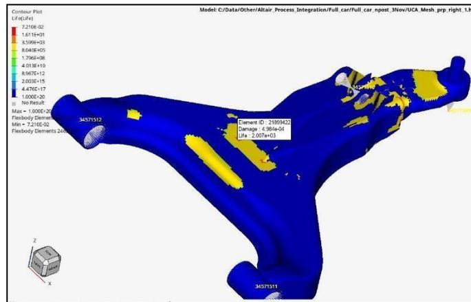
Fig 25. Npost fatigue analysis results for Wheel force
