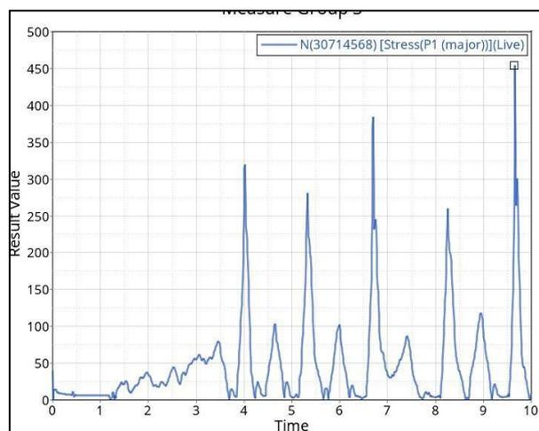
Fig 24. Stress plot for N Post wheel Force load case
