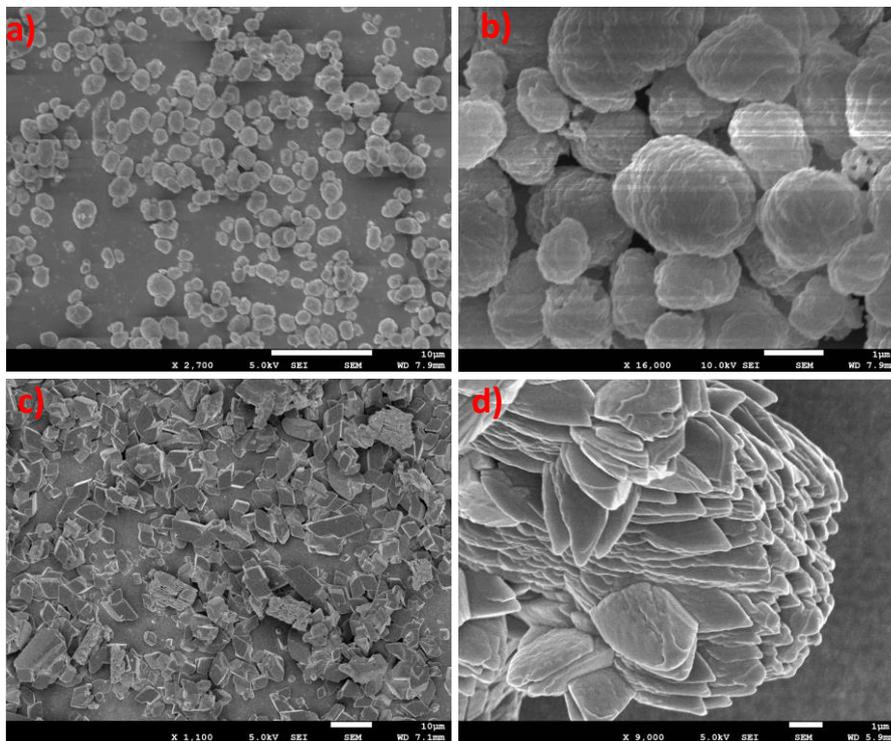
**Fig. 5. 6** FESEM image (a-b) CR(1:1), (c-d) CR(1:2) powder samples.
