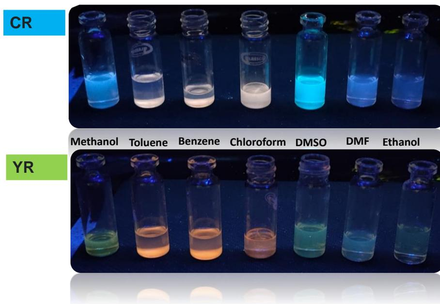
**Fig. 5. 10** Test of solubility of CR and YR in different solvents for coating optimization.
