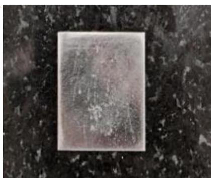
**Fig. 6. 2** Polished sample of Mild Steel.
