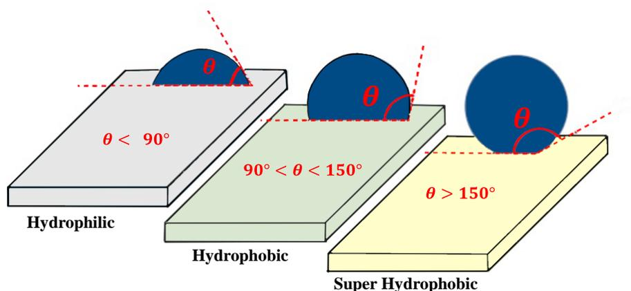
**Fig. 1. 2** Nature of surfaces based on contact angle.
