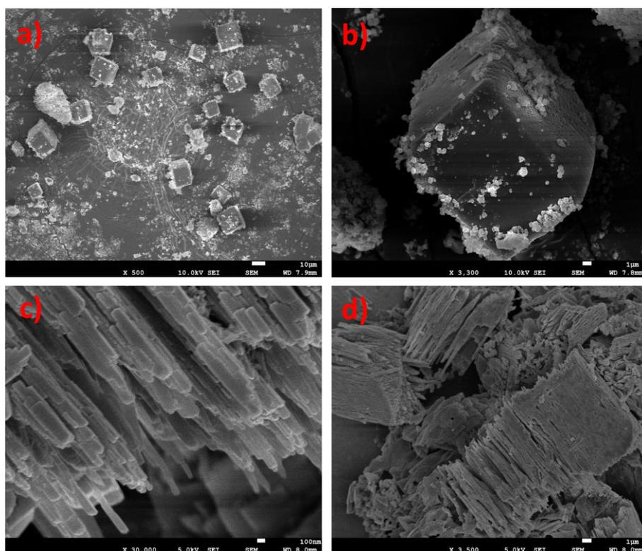
**Fig. 5. 7** FESEM image (a-b) YR (1:1), (c-d) YR (1:2) powder samples.
