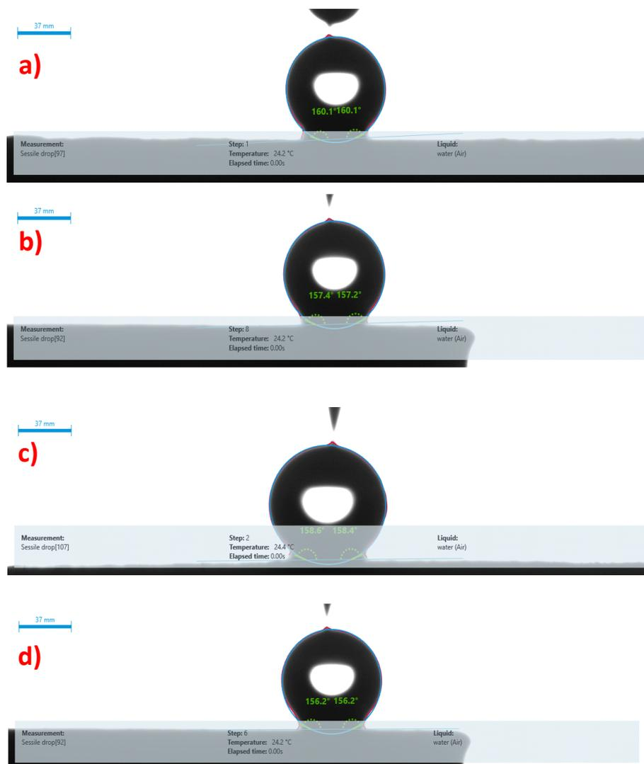
**Fig. 5. 11** Contact angle measurement of CR and YR coatings a) YR (1:1), b) CR (1:1), c) CR (1:2), d) YR (1:2).
