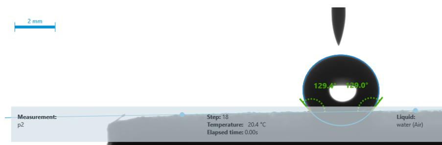
**Fig. 5. 2** Contact angle measurements of different coating samples of BCD powder.
