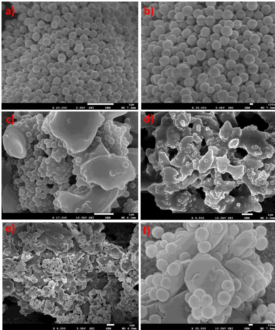
**Fig. 5. 8** FESEM image a-b) PVDF coatings, (c-d) PVDF with CR (1:1), (e-f) PVDF with CR (1:2) powder samples.
