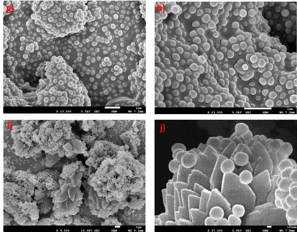
**Fig. 5. 9** FESEM image (g-h) PVDF with YR (1:1), (i-j) PVDF with YR (1:2) powder samples.
