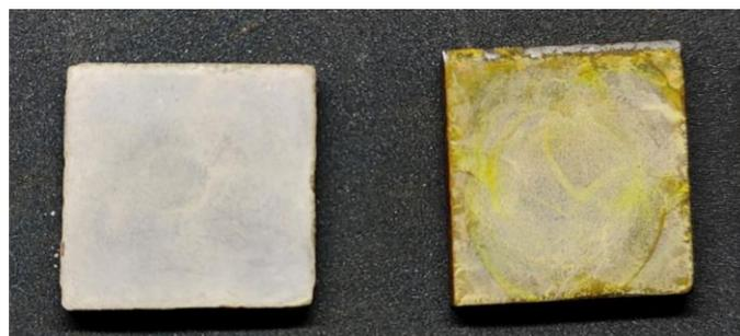
**Fig. 6. 3** Superhydrophobic coatings prepared using CR and YR carbon dots.
