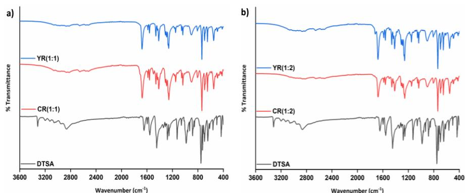
**Fig. 5. 3** FTIR data of CR and YR powders under different molar precursor concentrations.
