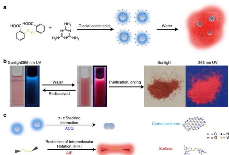
**Fig 2. 1** a) The generation of H-CD monomers and their conglomerates is being investigated, with emphasis on the disulfide bond present in the dithiosalicylic acid molecule, which is visually marked in yellow. b) Photographs depicting the luminescence principle of the H-CDs' dual-switch mode. c) The principle of fluorescence and the suggested configuration of the core and surface of H-CD are depicted, with the glowing edges corresponding to the hue of their fluorescence [13].
