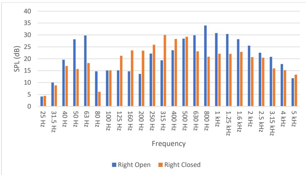
**Fig. 4.4 Frequency v/s SPL spectrum in 1/3 octave band in RIGHT direction (OFF)**
