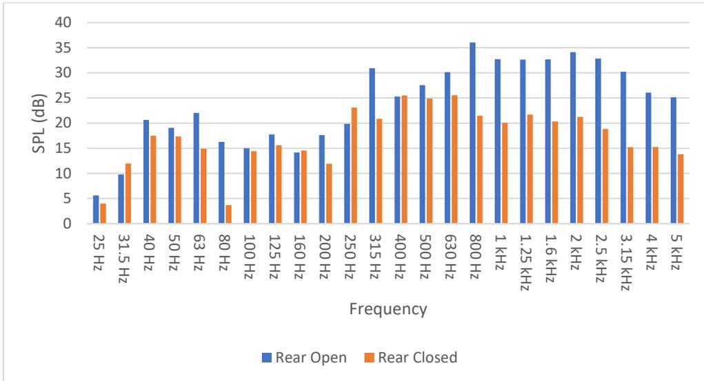
**Fig. 4.3 Frequency v/s SPL spectrum in 1/3 octave band in Rear direction (OFF)**
