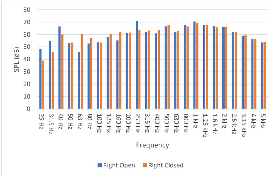
**Fig. 4.12 Frequency v/s SPL spectrum in 1/3 octave band in RIGHT direction (Working)**
