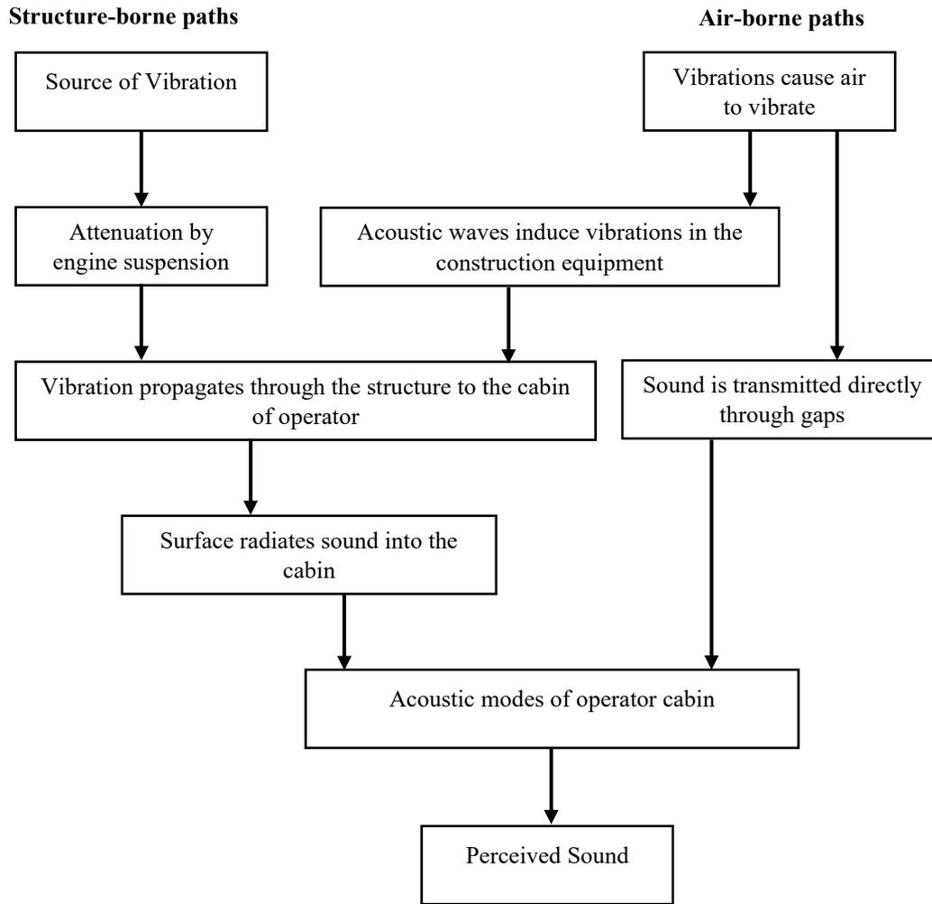
**Fig. 1.3 Structure-borne and air-borne paths of sound transmission**
