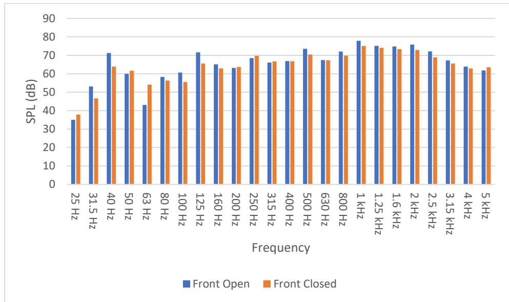
**Fig. 4.9 Frequency v/s SPL spectrum in 1/3 octave band in FRONT direction (Working)**
