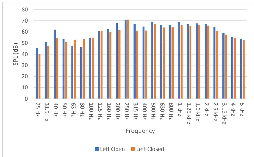
**Fig. 4.10 Frequency v/s SPL spectrum in 1/3 octave band in LEFT direction (Working)**
