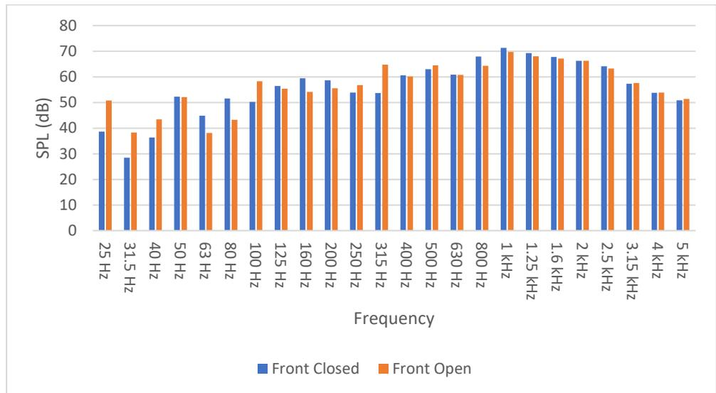
**Fig. 4.5 Frequency v/s SPL spectrum in 1/3 octave band in FRONT direction (ON)**
