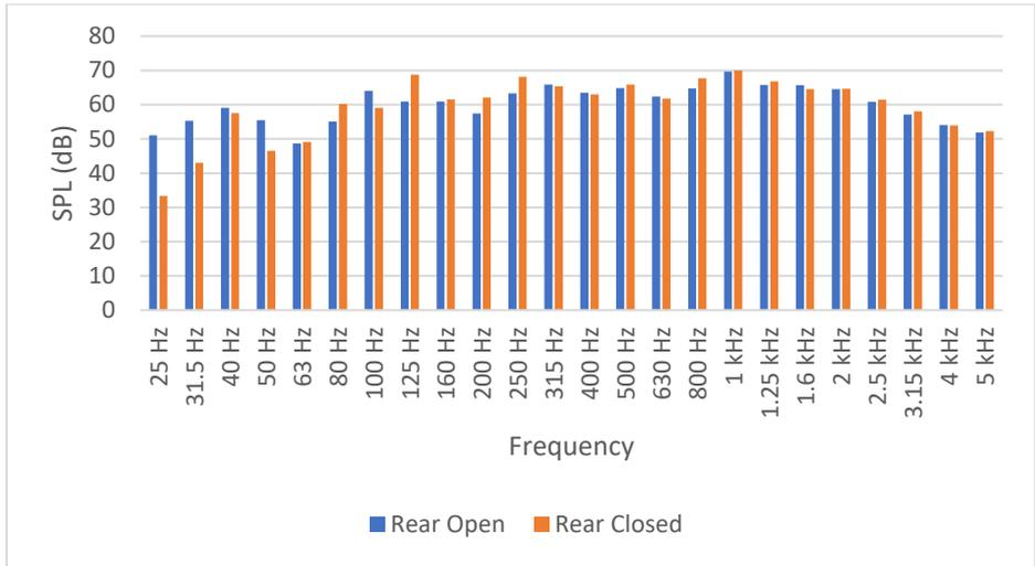
**Fig. 4.11 Frequency v/s SPL spectrum in 1/3 octave band in REAR direction (Working)**
