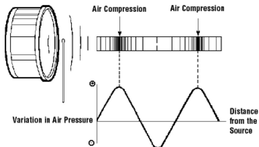
Fig. 1.1 Generation of sound waves [1]
