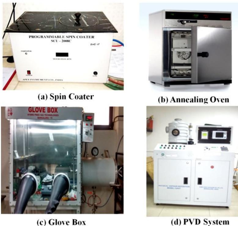
**Fig. 2.12: : Instruments used for the fabrication of devices**
