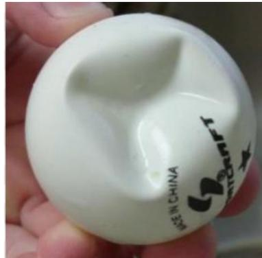
**Figure 1.2.** Snap through buckling of thin-walled table tennis ball.
