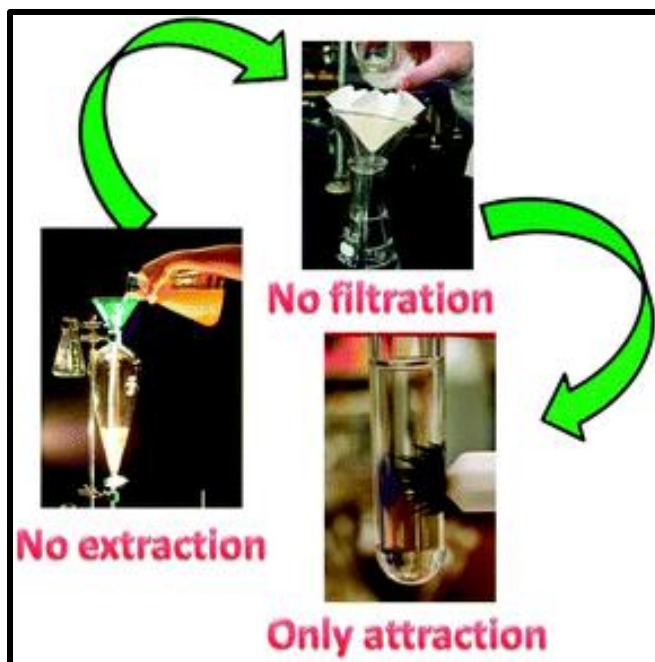
Figure 1.5. Bimetallic catalyst separations using external magnet.[31]
