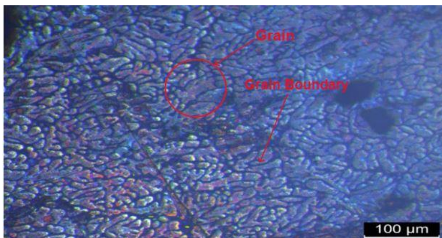
Figure 441. Microstructure Obtain Through RMP (Set-2, 12 TONS).
