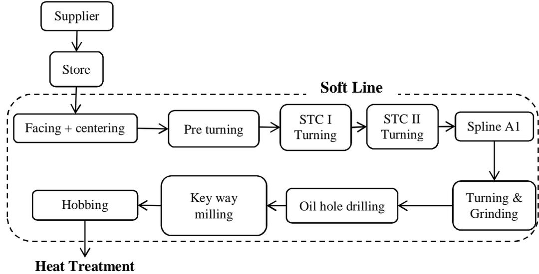
**Figure 4.2** Process flow of main shaft
