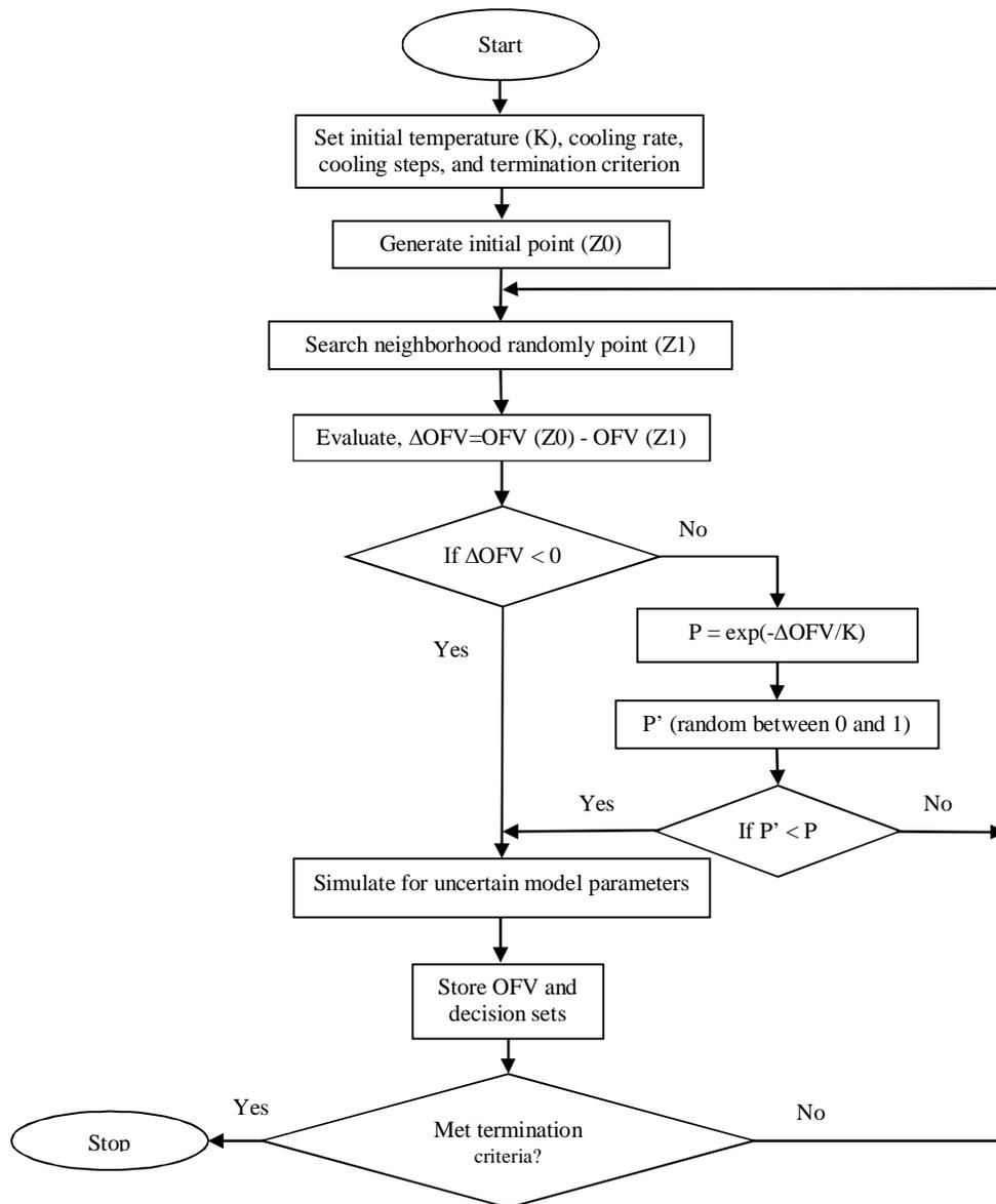
**Figure 3.7** A flow chart of simulation-based Adaptive Thermo-statistical Simulated Annealing
