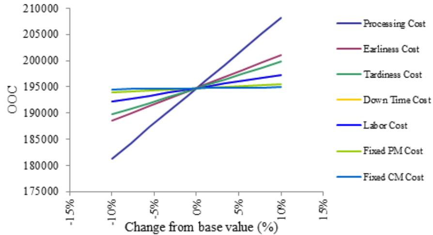
**Figure 3.3** Mean of OOC vs Percentage change of cost parameters
