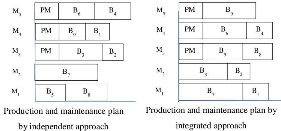
**Figure 3.4** Comparison of production and maintenance plan obtained from independent approach and integrated approach
