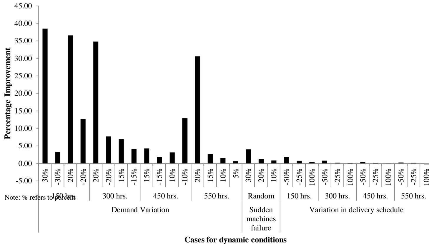
**Figure 5.6** Performance of the proposed approach over centralized approach (disturbance is adjusted at last) under dynamic conditions
