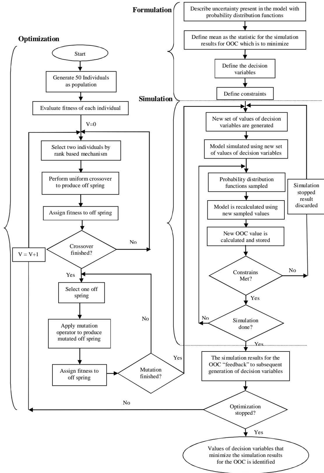
**Figure 3.1** A flow chart of Monte Carlo simulation-based genetic algorithm
