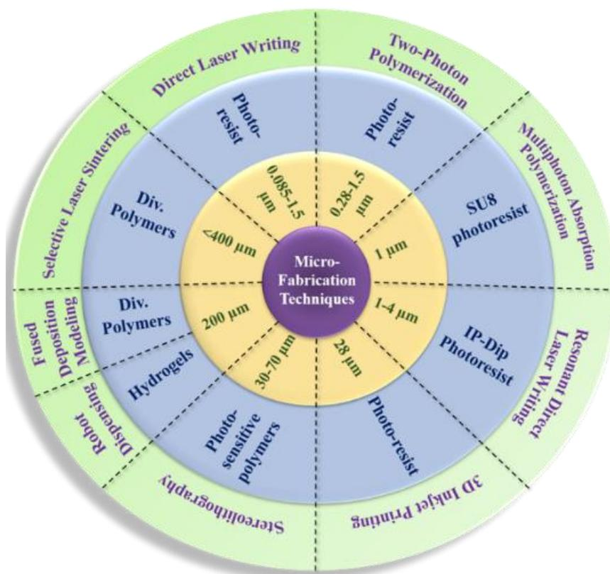
**Figure 1.4 Micro-Additive manufacturing Techniques. [4]**
