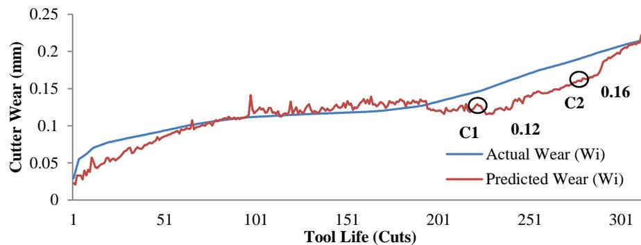
Fig. 3.3. Actual vs. predicted wear from online wear prediction model.
