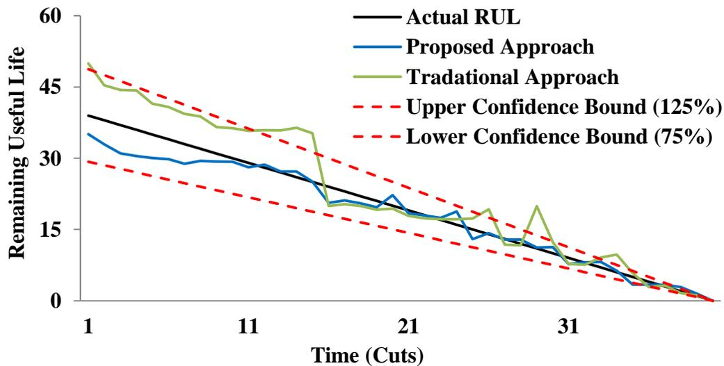
Fig. 5.12. Comparison with confidence bounds on the actual and predicted output under the scenario I.
