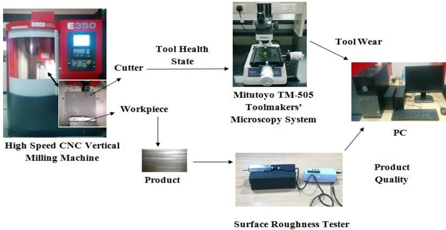
Fig. 4.1. Experimental setup.
