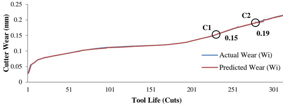
Fig. 3.4. Actual vs. predicted wear from semi-offline wear prediction model.
