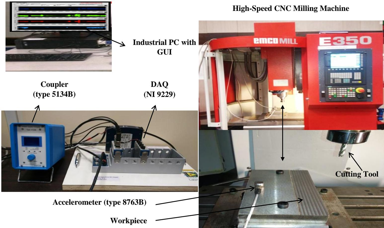
Fig. 5.6. Experimental platform.
