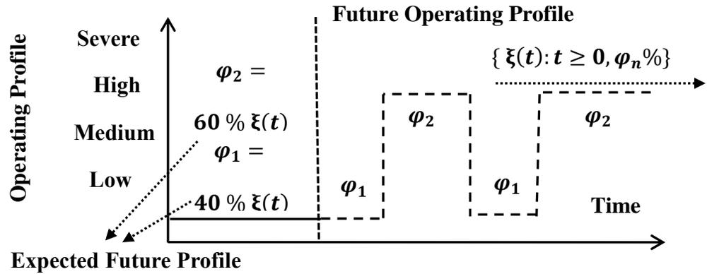
Fig. 5.5. Expected but fluctuating dynamic operating profiles.
