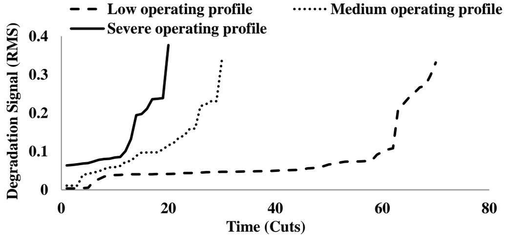
Fig. 5.1. Real-life degradation signals under various operating profiles.
