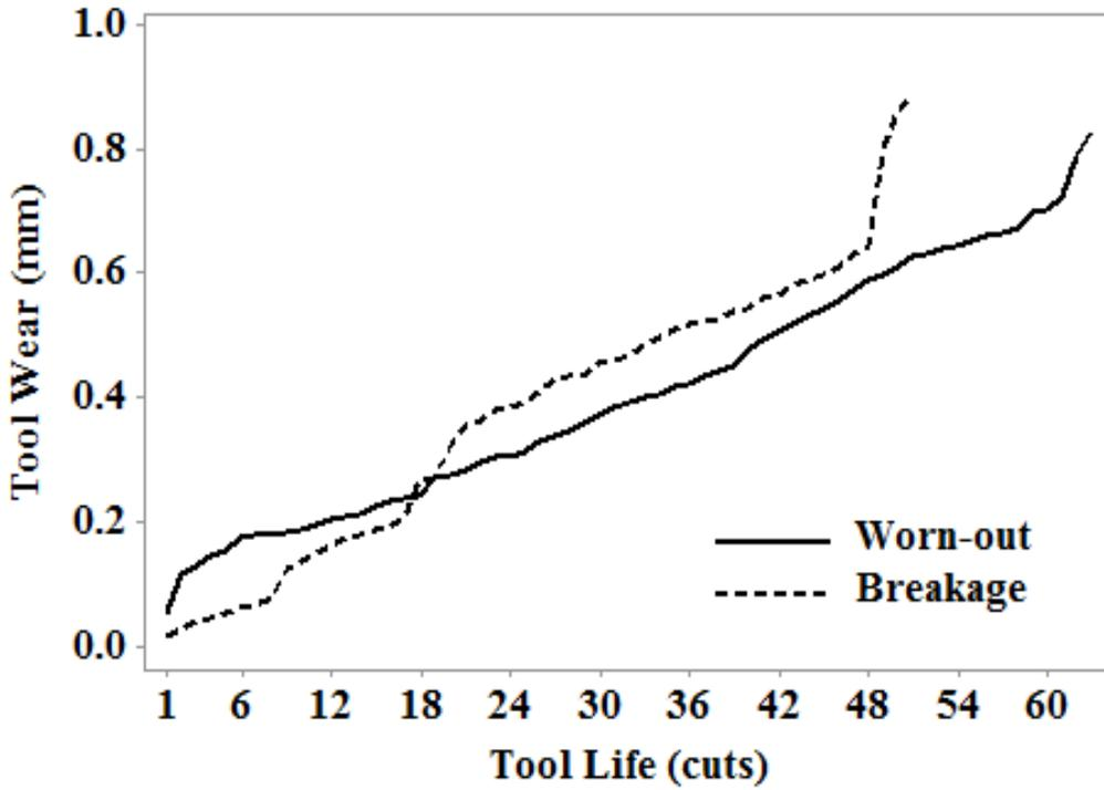
Fig. 4.2. Wear behaviour vs. tool life.
