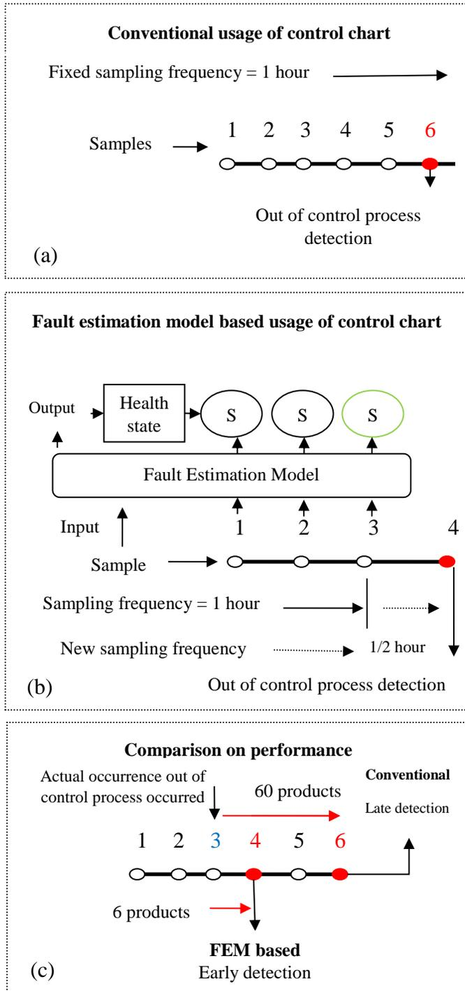
Fig. 6.2. Illustration of conventional and fault estimation based process monitoring and quality control policies.
