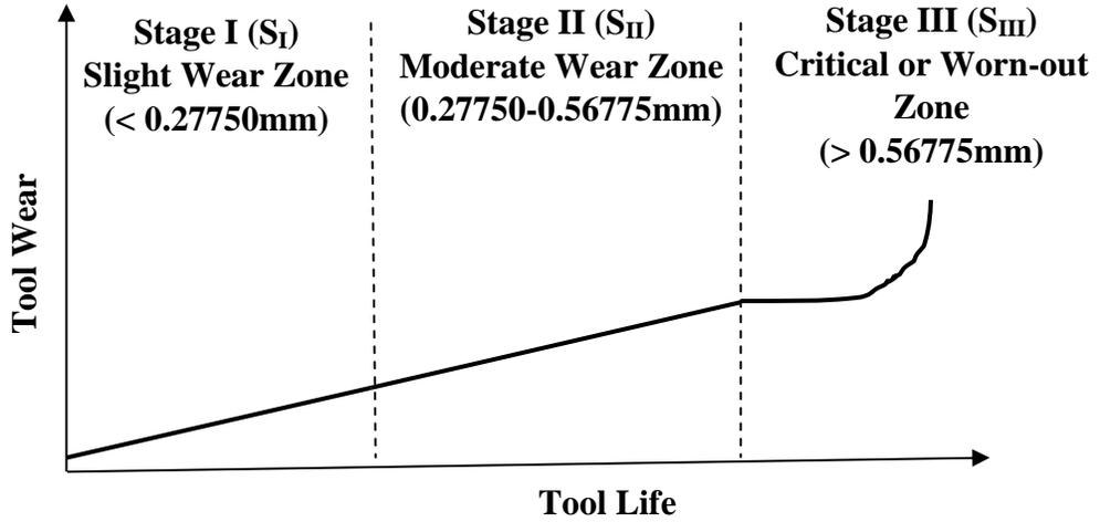
Fig. 4.5. Tool health states as a function of tool life.
