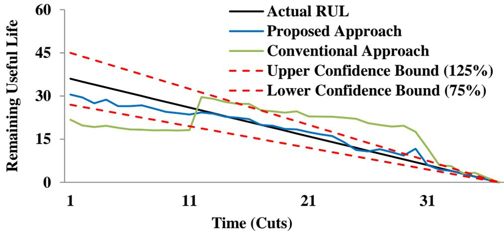
Fig. 5.13. Comparison with confidence bounds on the actual and predicted output under the scenario II.
