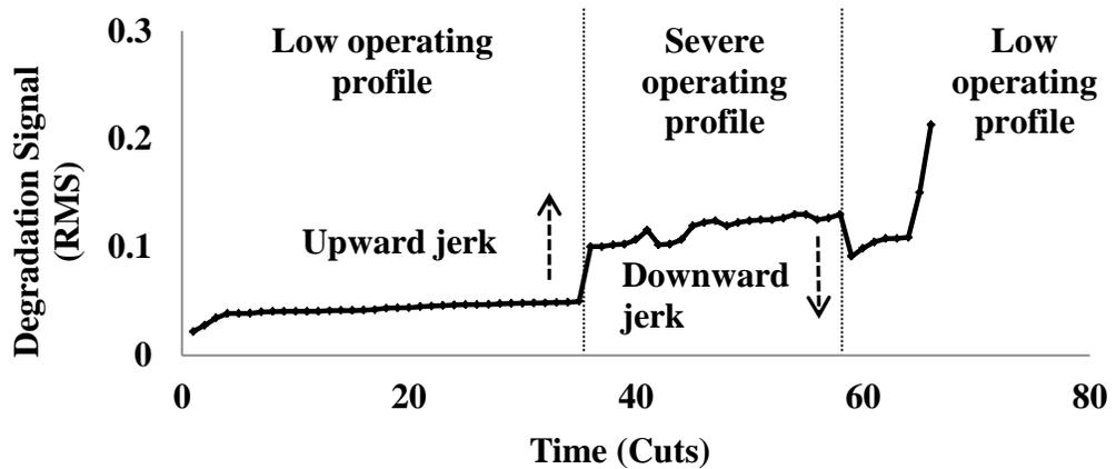
Fig. 5.2. Real-life degradation signal in time-variant operating profiles.
