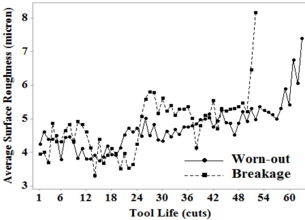
Fig. 4.3. Average surface roughness behavior vs. tool life.
