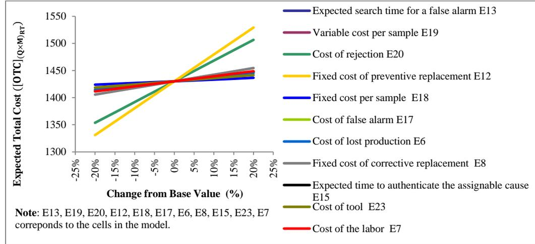
Fig. 6.5. Expected total cost vs. percentage change of the model parameters.
