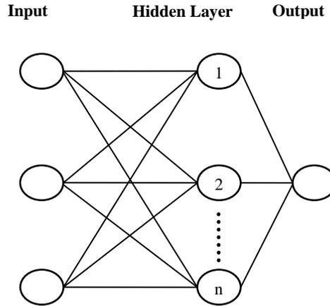
Fig. 3.2. Architecture of FFBP neural network.
