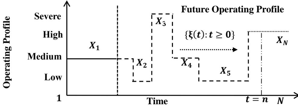
Fig. 5.4. Randomly-varying dynamic operating profiles.
