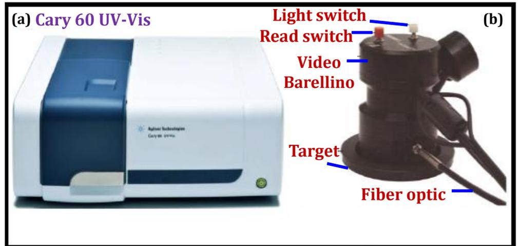
**Figure 3.7:** Experimental set up for diffuse reflectance measurement (a) Carry 60 UV-Vis spectrometer, (b) an integrating sphere attachment to detect diffuse reflectance.
