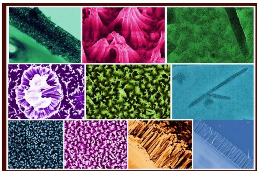
**Figure 1.2:** Various morphologies of Si NSs fabricated using MIE.
